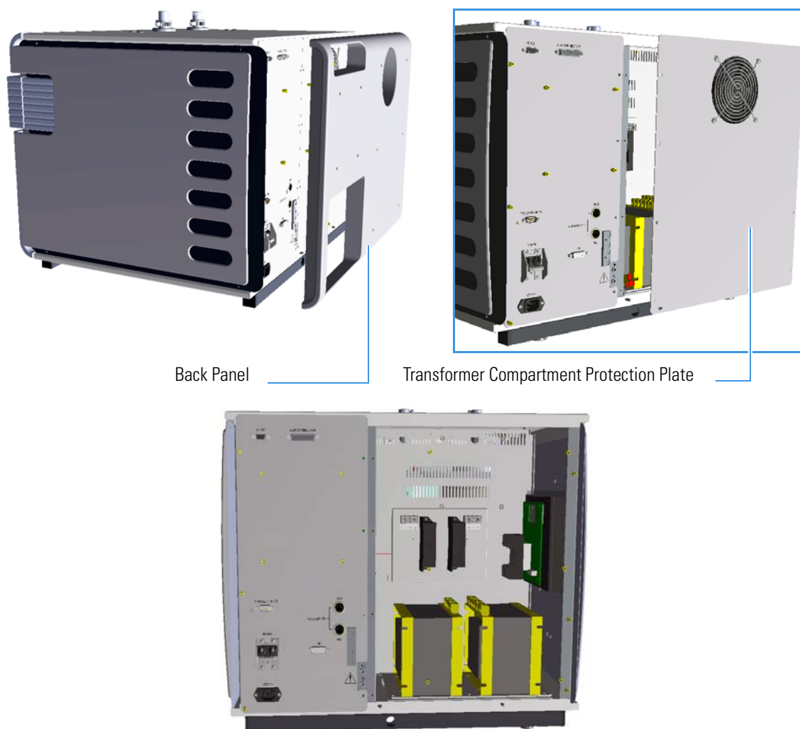
Figure 23. Accessing the Transformer Compartment
