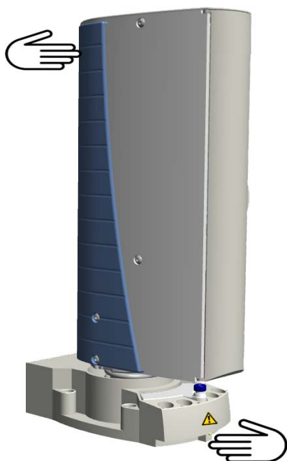
Figure 68. How to Lift and Carry the Sampling Unit
