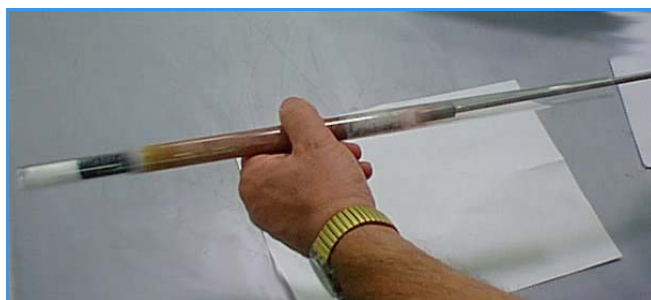
Figure 134. Removing the Filling Material from a Quartz Reactor
