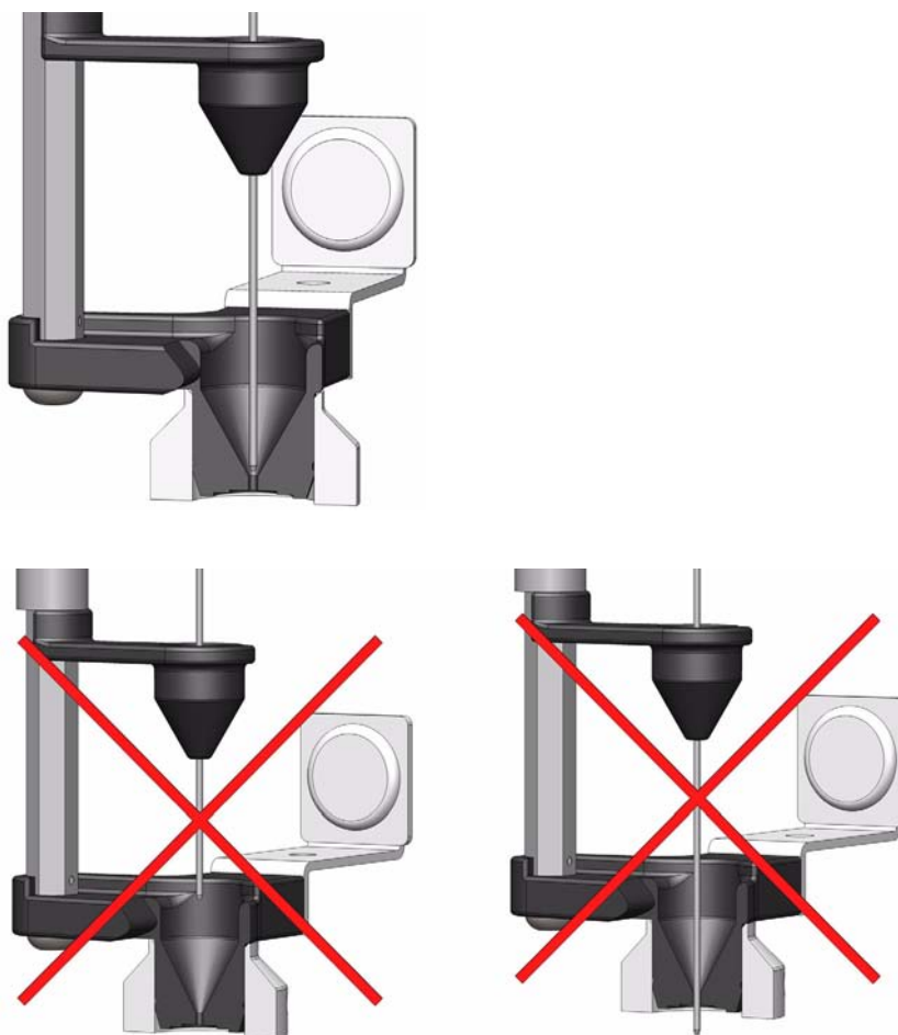
Figure 48. Correct and Incorrect Position of the Syringe Needle Tip
