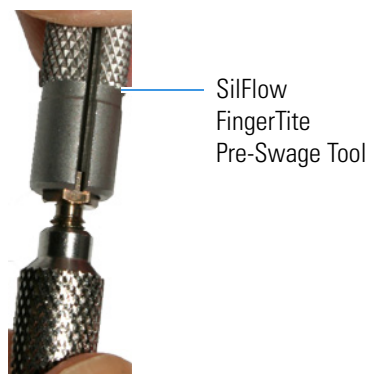
Figure 21. Swaging the Ferrule Using the SilFlow FingerTite Tool
