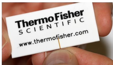
Figure 19. Cutting the Tubing with the Scoring Wafer
