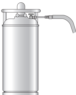
Figure 16. Liquid Nitrogen Tank Configuration
