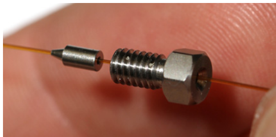
Figure 384. Positioning the SilFlow Nut and SilFlow Ferrule Correctly on the Tubing
