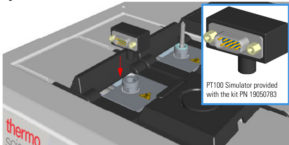
Figure 437. PT100 Simulator Installation
