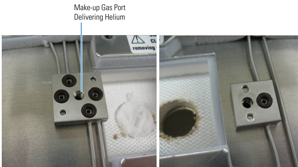
Figure 484. Confirming Presence of O-rings
