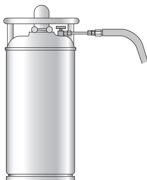
Figure 24. Liquid Nitrogen Tank Configuration
