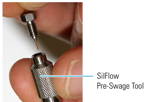
Figure 387. Inserting the Column and Ferrule into the SilFlow Pre-Swage Tool
