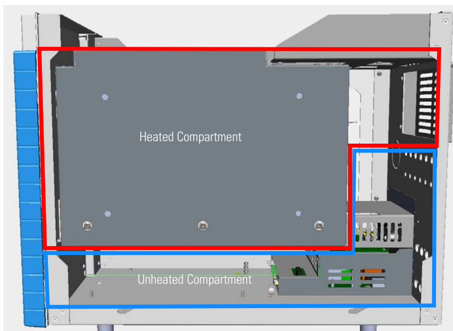
Figure 11. TRACE 1310 Auxiliary Oven Compartments
