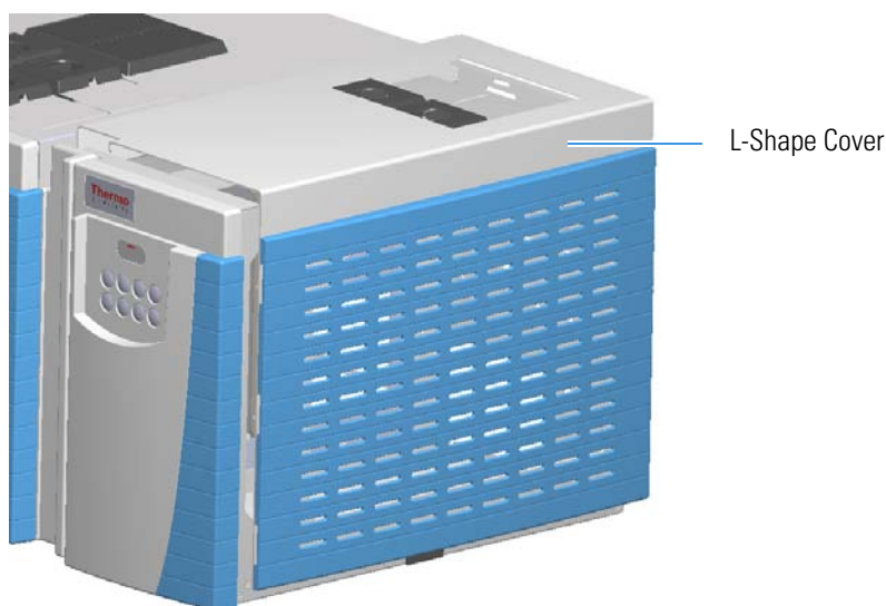
Figure 25. TRACE 1310 Auxiliary Oven L-shape Cover
