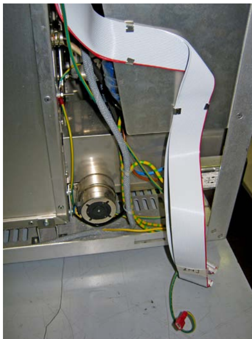
Figure 150. Fixing INJ and DET Auxiliary Oven Flat Cables (2)
