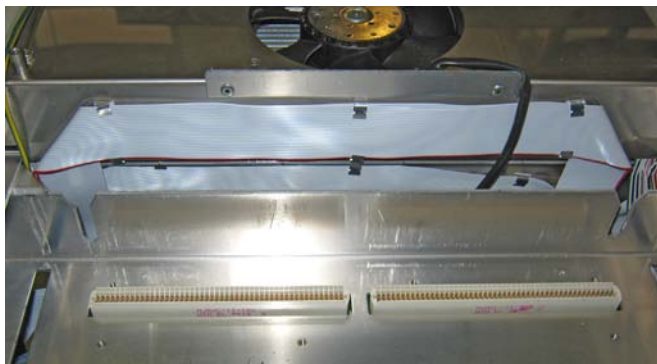
Figure 149. Fixing INJ and DET TRACE 1310 Auxiliary Oven Flat Cables (1)
