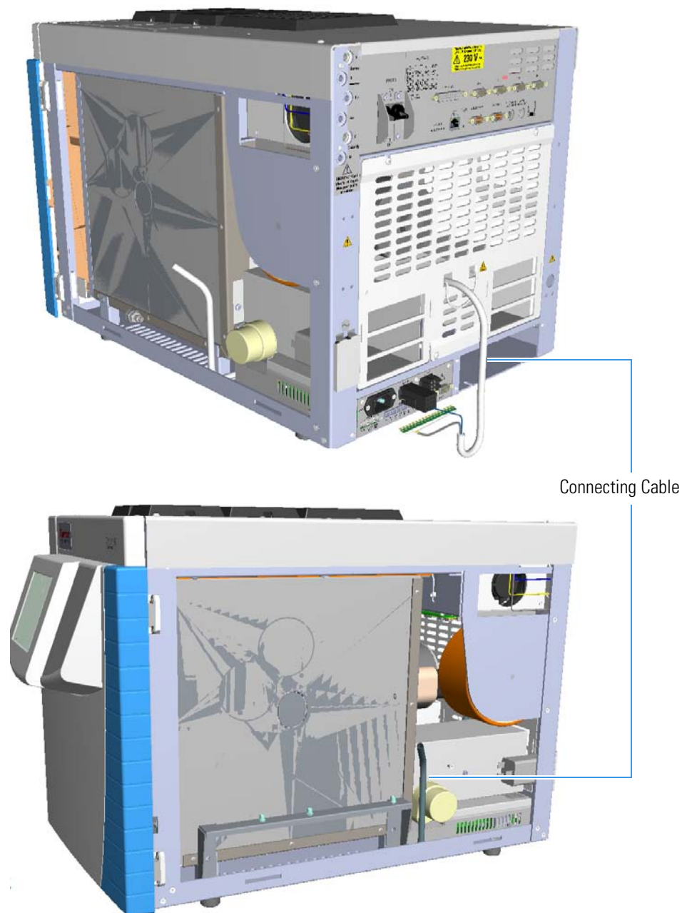
Figure 48. Connecting Cable Installation
