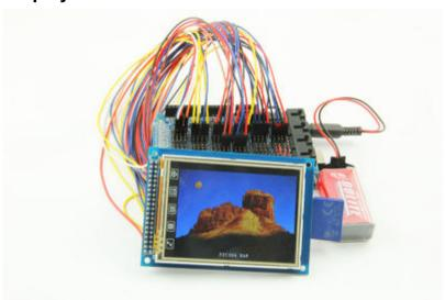
The UTFT library is required to be installed to get this screen model display. This library is especially designed for 3.2" TFT LCD screen using 16 bit mode. The library require the following connections.
