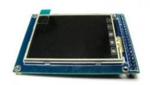
HY-TFT320 is a 3.2 inch TFT LCD Screen module, 320\*240 (resolution), 65K color, 40pins interface, not just a LCD breakout, but include the Touch screen, SD card. So it's a powerful extension module for your project.
