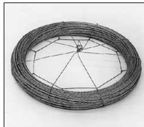
3. Twist at least two inches of the legs together until the wire cage is tight.
