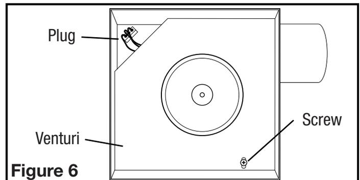
**NOTE:** If the fan motor plug is connected to the fan housing receptacle, unplug so the blower assembly can be completely removed.
