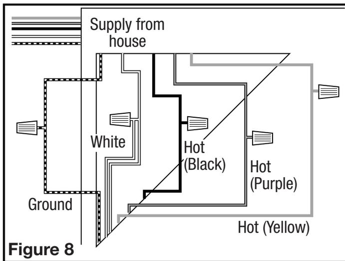
**NOTE:** The fan's receptacle wires might need to be pulled outside compartment for connection. Only pull the three loose wires outside of compartment. Additional wires will be present.
