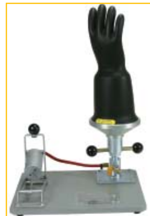
G2 with inflated glove ready for inspection.
