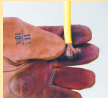
Embedded Wires: Inspect for embedded wires or metal shavings that could puncture rubber gloves.
