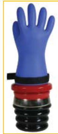
G100 with inflated lo-volt glove ready for inspection.
