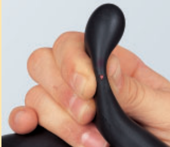
Snags: Damage shown is due to wood or metal splinters or other sharp objects.
