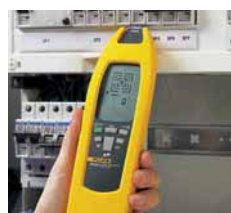
Location of fuses/breakers and assignment to circuits
