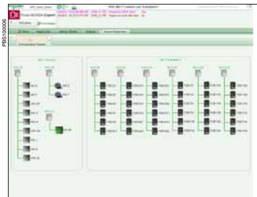
System Supervision displays such as this let the user see the real-time status of all devices and provide detailed information for best decision making.
