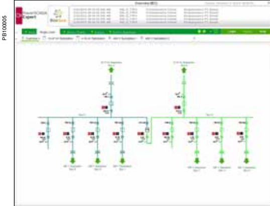
Monitor the whole communications network. Connect to switches, IEDs, RTUs, control and monitoring devices. Extract values for dynamic power and energy readings.
