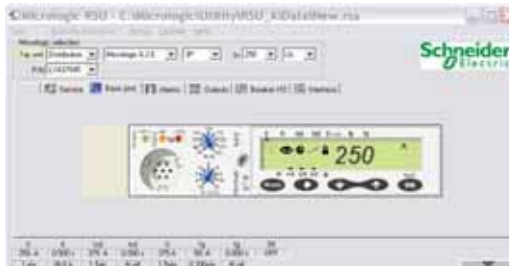
RSU mini-supervision screen for current measurements.
