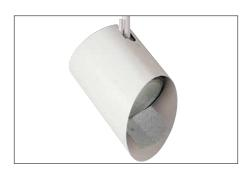
ProSpec Wall Washers feature an asymmetrical spread lens and an anodized aluminum kick reflector to distribute light evenly from ceiling to floor. The kick reflector assembly can hold one accessory and be removed from the front for relamping. ProSpec's Tru-Lock™ aiming mechanism allows simultaneous locking of both horizontal and vertical positions. Ring Wall Washers feature highly adjustable yoke mounting.
