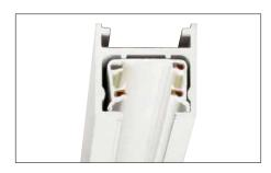
Advent double-circuit track allows for separate control of the Lytespots on the same track. It can be surface or stem mounted on ceilings, and mounted vertically or horizontally on walls, in straight runs or patterns. It can be field cut to the desired length. Total capacity is 40 amps when supplied by a single phase, 120/240V three-wire branch circuit.
