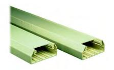
PAN-WAY T-70 Surface Raceway is a multichannel system that allows you to route copper, fiber optic and/or power cabling in one raceway. Electrical and communications devices can be mounted inside the raceway to provide a clean, attractive solution with maximum security.
