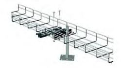
Attaches to round or square access floor posts. Use with FAS Profile for support of up to 12 in. Cablofil wire cable tray. Each UFCN comes with four mounting bolts and nuts. Standard finish: Electro Zinc coated for superior corrosion resistance. Other finishes include: Pre-Galvanized (PG), Hot-Dipped Galvanized (GC), Black Painted (BL) and Custom Painted (PE).
