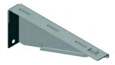
Use to support a wire-mesh cable tray pathway along a wall. Installation requires two 3/8 in. lag bolts and two flat washers for plywood backer boards or two 1/4 in. hex cap bolts, two flat washers and two appropriate anchors for concrete walls (ordered separately). Tray attaches to the Triangle Support Bracket with two splice washers from the Splice Washer & Bolt Kit or use the fold-over tab at the end of the bracket to secure the tray. Manufactured from steel. Finish: pregalvanized
