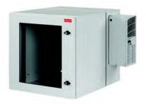
PROTEK Air-Conditioner Packages provide cool air to internal equipment when high ambient air temperatures exist (up to 130°F). A/C packages include an 800 Btu indoor/outdoor air conditioner that operates on 115 V AC with 5-15P plug.
