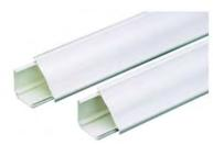
PAN-WAY Cove Raceway is a two-piece multichannel raceway, which has the appearance of architectural molding that allows you to route, conceal, protect and terminate power and/or data cabling. This aesthetically pleasing and unique design softens the horizontal angles between wall and ceiling or the vertical angles between two walls. Cove Raceway may be painted to match any décor.
