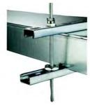
The SN Series Nut is an innovative new solution for supporting loads on threaded rod. The SN Series Nut is easy to install and can be positioned instantly on threaded rod at any location, helping to reduce installation time. Simply open the nut and insert it on the threaded rod where needed. Then twist it to close and tighten with a wrench.
