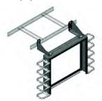
The PatchRack is a miniature two-post rack that can be attached to runway to save rack-mount space by placing patch panels or interconnect equipment above the rack or cabinet. Use to create a zone network in a data center. Attaches to all CPI cable runway, but optimized for 3/8 in. wide by 1 1/2 in. high side stringers or cross members.
