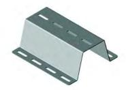
Use to support wire-mesh cable tray from the floor under an access floor. Attaches to the floor with 1/4 in. hardware or adhesive. Tray attaches to the Under Floor Support with a splice washer from the Splice Washer & Bolt Kit. Under Floor Supports can be used in pairs to support wider trays. Manufactured from steel. Finish: pregalvanized
