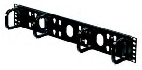
Constructed of a steel panel with PVC D-Rings attached. Mounts to 19 in. rack or cabinet. Includes mounting screws. There is an optional snap-on cover.
