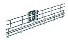
Attaches tray up to 4 in. wide to walls, cabinets or machinery. The fold-over tabs secure the tray without additional hardware. Slotted mounting holes make for adjustable installations. Also available in Hot-Dipped Galvanized (GC), Stainless Steel (316L), Black (BL), and Custom Painted Color (PE) finishes.
