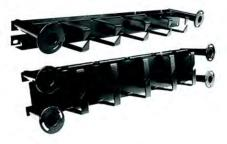
19 in. Horizontal Wire Management Panels for use on CPI racks or QuadraRacks when equipped with the VCS Vertical Cabling Section or for use within any CPI Cabinet System. CPI recommends planning 1U of cable management for every 2U of connectivity.
