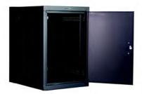
The WD series offers configurations ranging from 24 in. to 36 in. in height, offering 11, 18 or 25 rack-mounted units (RMU) of space. A simple finger pull/latch mechanism located inside the enclosure opens the 25.75 in. deep center swing section. The two pairs of 12-24 mounting rails are fully adjustable. The unique hinge system allows for removal of the rear section for easy installation. Casters are also available to make the WD free-standing as well as to be able to hold extra weight.
