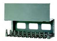
Manage cables on switches with vertical cords, curved cable management fingers support cables as they transition to the vertical pathway, can be used to create cable pathways for routing cable. Steel hinged cover provides easy access to pathway, pass-through holes on top and back of manager, mounts to 19 in. EIA racks and cabinets, mounting hardware included.
