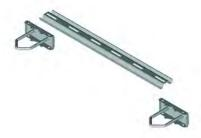
Use to support wire-mesh cable tray from the ceiling with a single 3/8 in. threaded rod. Tray attaches to the Center Support Bracket with two splice washers from the Splice Washer & Bolt Kit or use fold-over tabs to secure the tray on all sizes except the 4 in. W version. Manufactured from steel. Finish: zinc electroplate
