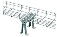
Use a single support assembly for tray widths up to 20 in. Use two supports for tray widths up to 24 in. Patented FAS-style attachment secures tray without nuts and bolts. Predrilled mounting holes make installations easy. Tray is supported independently of raised floor systems. 4 in., 6 in., 8 in. and 12 in. heights now available in widths up to 20 in. Contact your local sales representative for further details.
