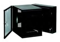
ACCESSPLUS II Cabinets provide security, equipment access, cooling and support for network and other 19 in. rack-mount equipment. The cabinet has three components: front door, center section and wall section. Double-hinged for easy equipment access; center section provides 19 in. rack mounting per EIA universal spacing and is accessed through the front door or swing the center section away from the wall section for rear access.
