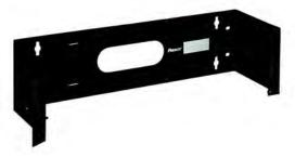
Mounts to wall or standard EIA 19 in. rack. Includes cable tie slots. Has standard 19 in. EIA hole spacing. Panel rotates from one side for easy access to cabling. Includes write-on labeling area and accepts 19 in. patch panels, horizontal cable managers and equipment.
