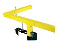
The FIBER-DUCT Routing System is a complete fiber optic-cable routing system that can be used for all fiber optic cabling installations. Used in telecommunications closets, equipment rooms or in approved under floor applications. The channel comes with standard mounting holes. The specially designed fittings feature a minimum 2 in. bend radius to protect fiber optic cables. The channel and fittings are made from V-O flame class-rated materials.
