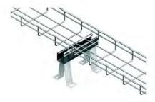
Use a single support assembly for tray widths up to 20 in. Use two supports for tray widths up to 24 in. Patented FAS-style attachment secures tray without nuts and bolts. Predrilled mounting holes make installations easy. Tray is supported independently of raised floor systems. Fiberglass strut design keeps cable pathway insulated from floor deck. 4 in., 6 in., 8 in. and 12 in. heights now available in widths up to 20 in. Contact your local sales representative for further details.
