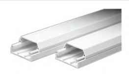
PAN-WAY T-45 Surface Raceway is a two-piece multichannel system used to route, protect and conceal data, voice, video, fiber optic and/or power cabling. The multidirectional hinged cover allows cable installation from either side. Hinged data and power brackets provide easy access for terminating outlets.
