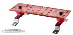
Manufactured of 1/4 in.-thick electrolytic tough pitch 110 alloy copper bar. Includes  $1\,1/2$  in. insulators and 1 in. off-set stainless steel mounting brackets. Includes one 1/2 oz. tube of antioxidant joint compound. Meets BICSI and ANSI/TIA 607 standards.
