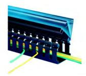
Type H Hinged-Cover Wide Slot Wiring Duct is a two-piece wide finger-design duct with dual-sided hinging cover that can be opened up to 100 degrees from either side of the duct. Ideal for applications that require frequent access, like in control-panel or cabinet wiring for equipment modifications or repair and in communications closets where moves, adds and changes are frequent.
