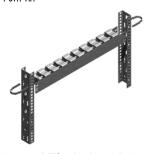
Crossbars secure the tray with FAS style tabs and the heavy-duty legs have multiple mounting holes for almost infinite height adjustments. The attachment clips secure installation to raised access floor legs. Each kit support includes one crossbar, two leg supports and two leg attachment clips. Kit components may be ordered individually. Other standard kit heights available: 3.5 in., 14 in. and 24.8 in.
