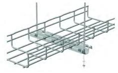
For trapeze-hung installations or use on walls, floors and cabinets. Patented FAS-style attachment holds cable tray secure without nuts and bolts. For trapeze-hung installations, use 4 in. longer profile than tray width. Can be used with up to 3/8 in. threaded rod. Also available in Hot-Dipped Galvanized (GC), Stainless Steel (316L), Black (BL), and Custom Painted Color (PE) finishes
