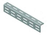
Use to support the end of wire-mesh cable tray against the wall. Installation requires two 1/4 in. lag bolts and two flat washers for plywood backer boards or two 1/4 in. hex cap bolts, two flat washers and two appropriate anchors for concrete walls (ordered separately). Tray attaches to the Wall-Mount Angle with two splice washers from the Splice Washer & Bolt Kit. Manufactured from steel. Finish: pregalvanized
