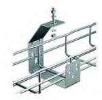
A part used for hanging 2 in. or 4 in. wide tray, with fold-over tabs that secure the tray without additional hardware. Threaded rod, nuts and washers sold separately. Also available in Hot-Dipped Galvanized (GC), Black (BL), and Custom Painted Color (PE) finishes.
