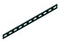
Use with splices from the Standard Splice Kit to create a more secure end-to-end connection between wire-mesh cable tray sections. Attaches to the side of the tray using three splice washers from the Splice Washer & Bolt Kit. Recommended for all trays that are 18 in. W or wider. Manufactured from steel. Finish: zinc electroplate
