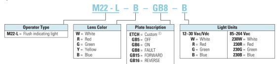
**Note:** Light unit should match color of lens. Use white light unit with yellow lens.
