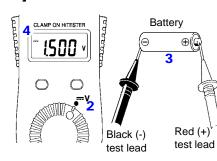
Reversing the polarity of the test leads displays a negative value.
