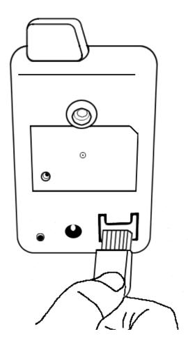
3. Plug the power adapter into a wall socket and connect the power connector to the power jack located at the back of the network camera.
