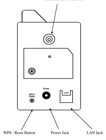
Camera Stand Connector: Connects to any standard tripod / camera wall holder. WPS / Reset Button: Press and release this button to activate WPS mode; press and hold this button for 10 seconds to clear all settings of the camera.
