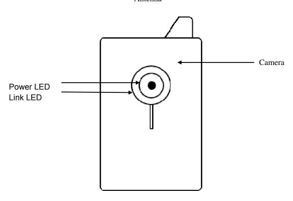
Antenna: Wireless network antenna Link LED: Indicates LAN / WiFi activity Power LED: Indicates system status Camera: Video camera with lens
