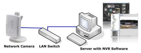
Example showing a network camera in a typical setup with an NVR recording solution.
