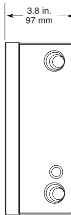
Side view of 8M Enclosure box showing depth
