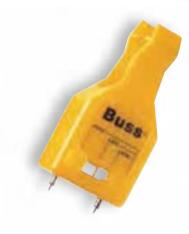
The **FT-3** combination fuse tester and fuse puller is designed for easy one-handed use. It tests glass and blade fuses in or out of the fuseblock. This continuity tester is for fuses in circuits up to 24V maximum. Light glows when fuse is good.
