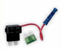
**BP/HHA** converts an ATC fuse circuit into two fusible circuits. It plugs into the fuseblock, and accepts two fuses to provide protection for the existing circuit and the add-on circuit (10 amp maximum).
