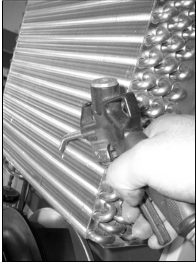
Fig. 79: Clean out the heat exchanger coil and compressor chamber using compressed air (2)
