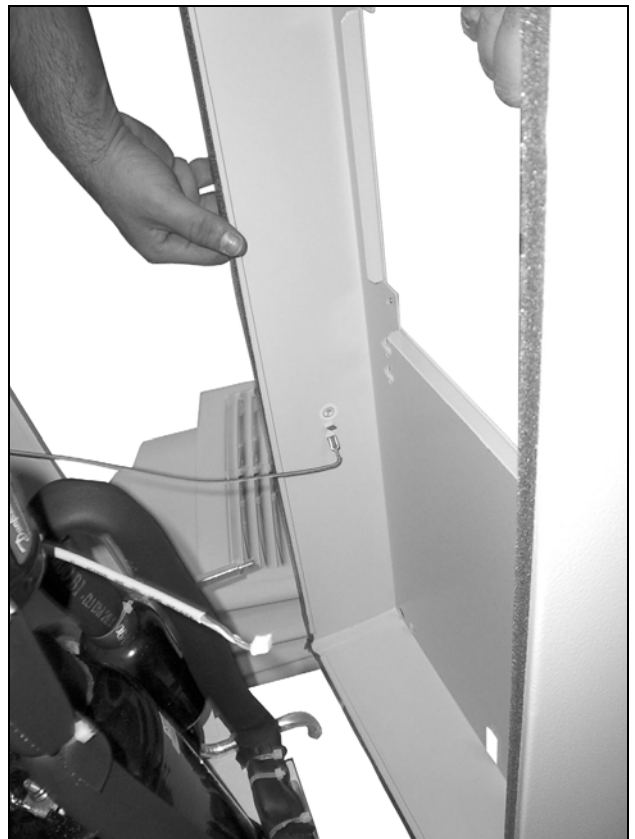
Fig. 76: Disconnect the earthing cable (1)
