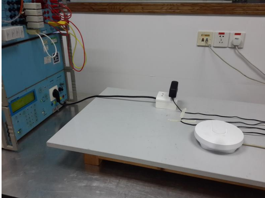
Continuous RF Immunity Test Set Up
