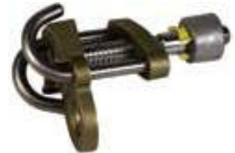
Wire Grip Grips conductor, has hole for block or line hook. WWL for grip is 1,000 lbs (454 kgs) at a 4:1 ratio. 3600 Opening min.5/16" max.7/8" 2 lbs (0.91 kgs) (7.9mm, 2.2cm) 3601 Opening min.1/2" max.1-1/2" 3 lbs. (1.36 kgs) (1.3cm, 3.8cm) Add suffix "U" for Universal, "Q" for Quick Change
