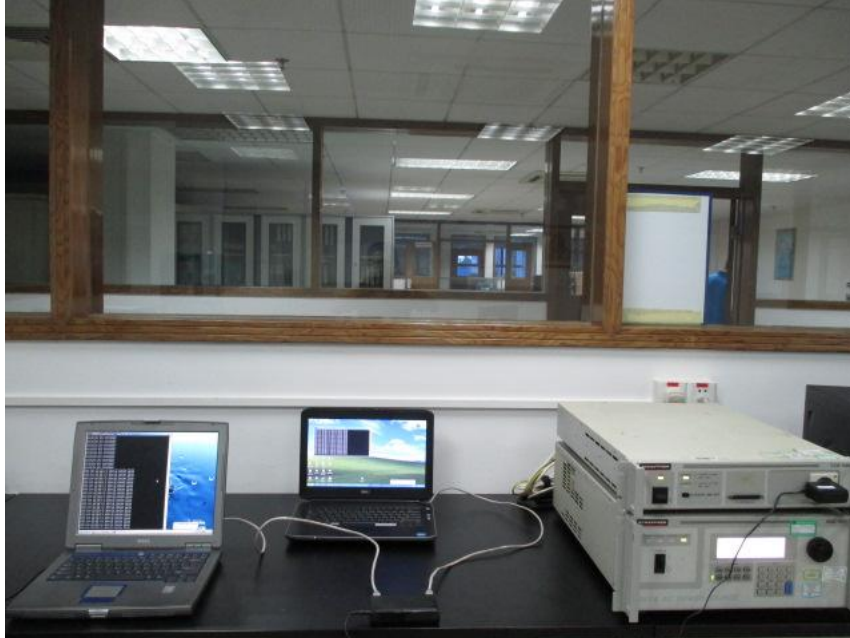
Harmonic Emissions & Voltage Fluctuations Test Set Up
