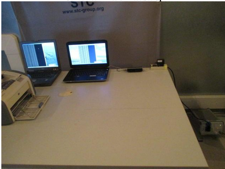
Conducted Emission Test Set Up
