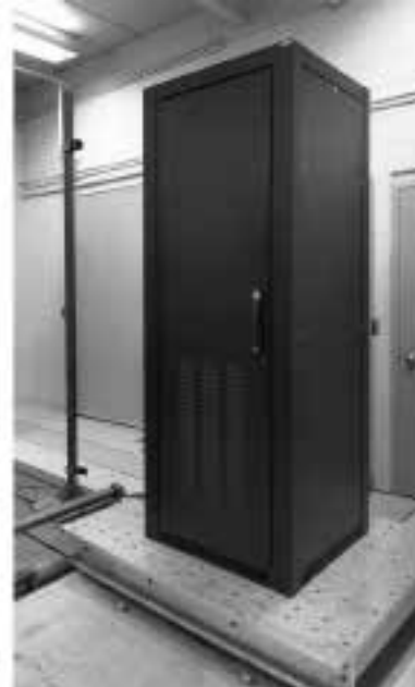
Enclosure mounted on shaker table
