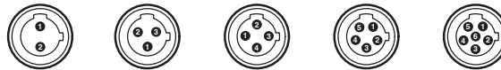
2-Pole Dual Key AC 3-Pole Dual Key AC 4-Pole Dual Key AC 5-Pole Dual Key AC 6-Pole Dual Key AC
