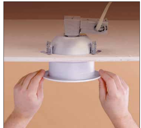
Exclusive mounting clips adjust to ceiling thickness with sliding teeth that grab hold of ceiling material and secure Cliclyte luminaire in position.
