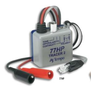
Permits technicians to identify the conductor within a bundle, at a cross-connect point or at the remote end. Can be used on twisted pair wiring (telecom, datacom, etc.), single conductors, coaxial cables, de-energized AC wiring and most other wiring.
