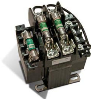
Fig 7. Eaton Cutler-Hammer control power transformer with built-on fuseholders. The transformer is protected by Cooper Bussmann fuses, primary by class CC type FNQ-R, and secondary by Midget Type FNM. Protective cover for fuses and terminals are available as accessories.
