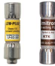
Fig 5. Left side fuse is rejection type class CC, right side fuse is a Midget fuse. The dimensions are the same for both types, 10,3x38,1 mm. One of the contact ferrules on the class CC fuse is equipped with a rejection key, in this case a tap. The design prevents installation of a Midget fuse in a fuseholder intended for class CC fuses.
