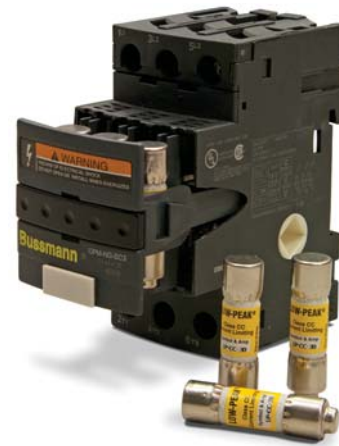
Fig 6. Cooper Bussmann Optima off-load fuse disconnecter with class CC type LP-CC fuses installed offers reliable protection for both motors and starters in a compact design.
