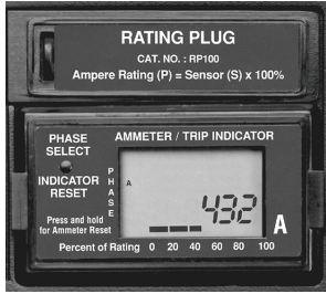
Combination Local Current Meter and Trip Indicator
