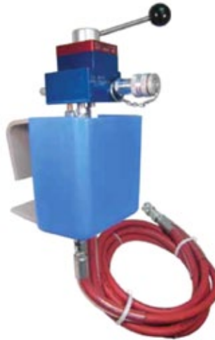
HFC30 Hydraulic Flow Control Valve Operates off of a vehicle's hydraulic circuit. It can accept a flow of up to 30 gpm and reduce it to a maximum of 10 gpm allowing the correct flow to the hydraulic tool.
