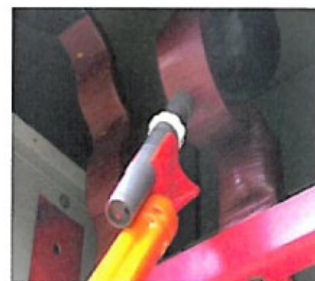
Typical applications of LVTs and LIVs include buss bar, overhead conductor, and underground cable voltage verification. Operational voltage ranges extend from 120VAC to 500KV.
