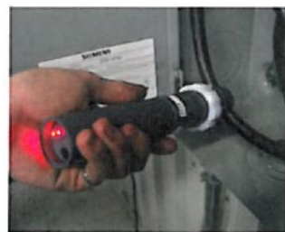
Typical applications of LVTs and LIVs include buss bar, overhead conductor, and underground cable voltage verification. Operational voltage ranges extend from 120VAC to 500KV.
