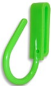
2402 - Handline Carrier A nylon handline carrier with a hole to easily secure it to the body belt with a bolt or zip tie, that will straighten when approximately 14-18 lbs of pressure is applied, allowing the hand line to pull free.
