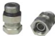
TE2066-6-8S Swivel Coupler 3/8" NPT Female to 3/4 x 16 O-Ring
