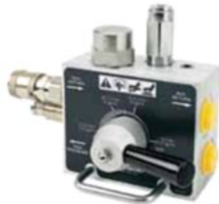
HFC30 Hydraulic Flow Control Valve Operates off of a vehicle's hydraulic circuit. It can accept a flow of up to 30 gpm and reduce it to a maximum of 10 gpm allowing the correct flow to the hydraulic tool.
