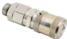
54925 Female Coupler 3/4"-16 SAE O-Ring, External Thread
