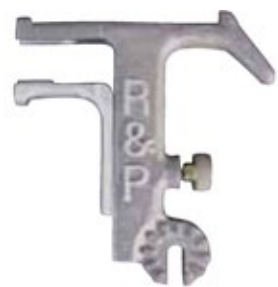
TESF1 Safety Finger A safety device for installing and removing cutout fuse barrels. The spring-loaded design firmly holds the fuse barrel in place and prevents it from falling. Fits standard 100 amp cutout fuse barrels.
