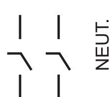
Three-wire SN, 120/240 Volts AC, No Fuse
