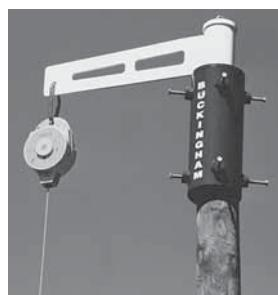
Adjustable to fit over a 9.5" diameter pole. Features center lifting eye and (8) bolts to secure pole. Limits arresting force to under 900 lbs. 5,400 lb anchor point. 10 minutes to install.
