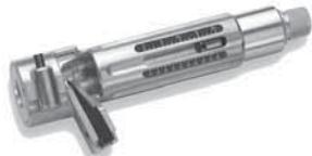
Features adjustable strip stop with rotary mechanism that eliminates the need for a hex wrench. Also includes adjustment window with inch and metric readings which allows for easy setting of stop for precise strip lengths. Strips lengths from 0.625" to 2.5".
