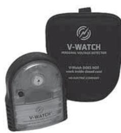
Detects presence of AC voltage electric fields surrounding electrical equipment. Designed to be worn on outside of clothing or other protective gear. Features audible/visual alarms that increase in frequency as device approaches energized equipment. Includes rugged protective housing, low battery indication, field replaceable 9V alkaline battery and built-in self-test system. Measures 3.5" x 2.88" x 1.25".
