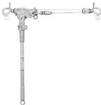
Features aluminum alloy frame, double interlocking pawl mechanism, breakable stress link overload indicator, self-lubricating bearings, steel latching hooks, and reversible 30" fiberglass handle. Open design allows visual inspection. 1-ton capacity (double line).
