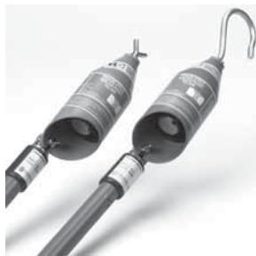
Designed to perform many of the existing functions of conventional voltmeter/phaser devices but is lighter weight and cordless. Consists of 2 units, a transmitter and receiver. Features built-in universal splines, clear in-phase/out-of-phase indicators, overhead probes, and carrying case.
