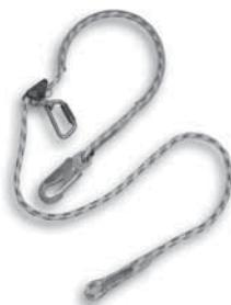
Fully adjustable positioning lanyard. Features length adjusting device specially designed with a 90 degree twist in the eye of the CAM for use with a line workers body belt. Also designed with full red core wear indicator, double locking rope snap and clear protective tube for maximum rope life. May be used as primary work positioning device.
