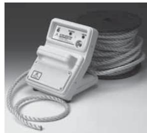
Designed to test hot line ropes, slings and straps for dielectric integrity at the time and location they are being used. For use on ropes from 3/8" dia to 1-1/2" dia. Features green and red LED, 8VDC rechargeable battery, and buzzer sound to alert defective rope.
