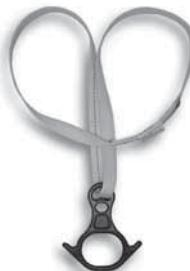
Designed to be girth hitched on a structure to aid in rescue of an injured victim. The strap is made from 1" yellow webbing and the Figure 8 is made from aluminum. Ears prevent rope from slipping down and knotting at the bottom of the Figure 8.
