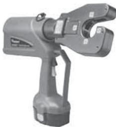
For use in tap, terminate and splice compression applications. Features ergonomic design, 360° rotating C-shaped head, trigger guard, audible pop-off valve and safety lanyard connection. Measures 17.6" L x 3.7" W x 13.9" H. Includes (2) 18V Ni-MH batteries, battery charger, lanyard and carry case.
