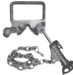
Provides protection for personnel in single point grounding applications. Features adjustable chain tightener with 36" of chain. Aluminum alloy construction. Accepts C- and duckbill grounding clamps. Tested for 43KA @ 15 cycles.
