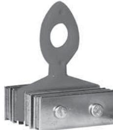
For use in eyelets of insulating blankets when covering energized portions in hard-to-cover areas like pad mounts, cubicles, switchboards and substations. Features four permanent floating magnets mounted between nickel-plated steel plates.
