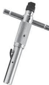
For use with 15 to 34.5 kV elbows. Prevents probe contamination and breakage. Reduces cross threading. Features removable T-handle, 1" steel drive, adjustable wrench, 3/8" square drive socket and Penta head.
