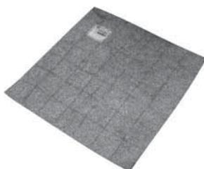
For use in underground padmount, transmission and distribution pole mount, and substation grounding grid applications. Hypalon marine fabric construction with high ampacity tinned-copper braid sewn into grid pattern. Copper braid connect to 6" termination stud on corner of mat. Weather resistant. Black.
