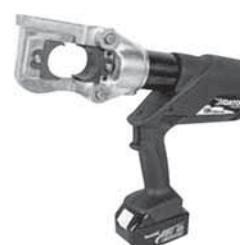
For use with U-style, 12 ton dies. Features two-speed pump, repeating retraction stop, LED light, 360° rotating head and pistol grip. 24,000 lbs. crimping force. Measures 16-1/2" L x 2-7/8" W x 14-1/2" D. Includes (2) 18V lithium ion batteries and carry case.
