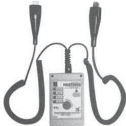
For testing new or trouble-shooting in-service transformers and capacitors. Verifies units are not shorted or open prior to energizing. Features magnetized back for hands-free operation, push button test feature, and (4) LED condition status lights. Includes 9V battery, storage case and instructions.
