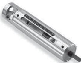
Ergonomic end stripping tool for 600V secondary cable, 1/0 AWG to 1000 MCM and is designed for use with a low or variable speed power drill. Reduces working time and effort on repetitive stripping jobs. Features adjustable strip stop with adjustment window.
