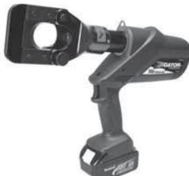
Designed specifically to cut ACSR, guy strand and ground rods. Features 18V lithium ion battery, retraction stop, LED, Two-stage hydraulic system, 350° rotating head, and one trigger to control all tool functions.
