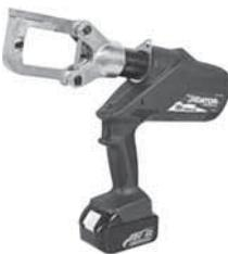
For use with W-style, 6 ton dies. Features two-speed pump, automatic retraction, repeating retraction stop, LED light, and pistol grip. 12,000 lbs. crimping force. Includes (2) 18V lithium ion batteries, 120V battery charger and carry case.
