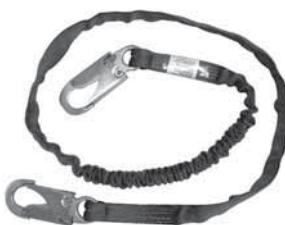
For use with full body harness having steel ring dorsal attachment. Features locking snap hook on both ends. Interior material stretches to reduce arresting force to less than 900 lbs.
