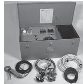
Designed to test substation rack of capacitors. Housed in case with handles. Requires 120-volt external power. Allows testing from 50 to 480 volts AC.
