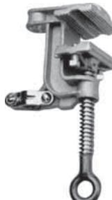
Features bronze body, serrated jaws, and bronze eyescREW with Acme threads. Drilled for 5/8"-11 UNC threaded ferrule. Fault current ratings: 43KA @ 15 cycles; 30KA @ 30 cycles.
