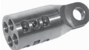
Designed to pull triplex or quadplex cables. 4 holes are sized for the cable conductors and each hole has three setscrews to clamp down on the cable. Includes (3) spare set screws and hex key.
