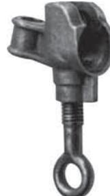
For use in industrial metalclad gear, substations and distribution applications where space is limited. Bronze alloy construction with tin-plated ball studs and silicone bronze lock-washer and nut. Tapped for 5/8"-11 UNC threaded ferrule. Fault current ratings: 43KA @ 15 cycles; 30KA @ 30 cycles. Meets ASTM Type I, Class A, Grade 5 specifications.
