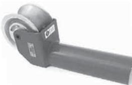
Designed with extra long tube section that goes inside the duct for greater stability. Features one half of a quick-disconnect coupling attached to spray nozzle that will direct the lubricant onto the cable as it is fed into the ducting.
