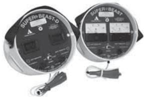
Indicates problems on secondary service and verifies condition of secondary conductors and associated connections. Isolates and identifies overhead or underground complaints on utility side and detects open neutral quickly and accurately. Meters register from 84-264 VRMS. Includes Digital meters, meter base adapter and bag.
