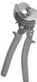
Designed to cut up to 954 ACSR and 1000 kcmil copper and aluminum. Features rugged steel blades and precision bi-directional ratchet mechanism for positive blade control.
