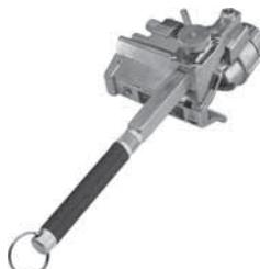
For use in removing PE, XLP, and EPR insulation from high-voltage power cables 1/2" to 1-3/4" OD. Features adjustable blade depth. Wedge blade installed; includes spare.
