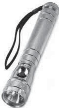
Constructed with anodized machined aluminum alloy and unbreakable polycarbonate lens. Corrosion and water resistant. Features 3.6V, 0.9A high pressure Xenon with (6) 100,000 LEDs (white). (3) C size alkaline batteries, not included.
