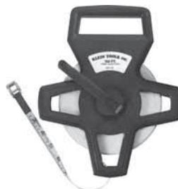
Woven fiberglass construction with polyvinyl chloride coating for resistance to moisture, oil and chemicals. Features black numbers and 1/8" graduations, red foot markings, and permanently attached end hook. Orange reel with handle for rewinding.
