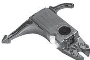
For use with hot sticks. Aluminum construction. Features pointed head for breaking ice or debris, notched straight arm to secure fuse, curved arm for hanging, LED light, high-low switch, and sealed borosilicate window. Waterproof to 1 meter. Requires (3) AAA alkaline or lithium batteries.
