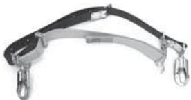
Key component of Jelco Pole Choker Fall Prevention Systems. The 1-3/4" wide yellow nylon strap squeezes the pole, the roller's teeth dig in to provide gripping force to prevent falling down the pole.
