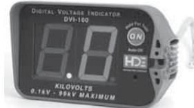
Single point instruments designed to read the voltage on a conductor up to 500kV line-to-ground. Features large LED readout and built-in universal spline for standard hotstick attachment.
