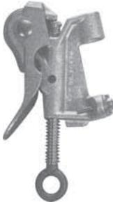
Aluminum construction with Acme-threaded bronze eye screw and stainless steel cable clamp for stress relief. Features smooth jaws. Main line range .162" min./1.16" max. 4/0 max. ground cable size. Fault circuit: 43KA @ 15 cycles; 30KA @ 30 cycles.
