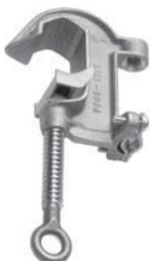
Features aluminum body, serrated jaws, and bronze eyescrew with Acme threads. Tapped for 5/8"-11 UNC threaded ferrule. Fault current ratings: 43KA @ 15 cycles; 30KA at 30 cycles.
