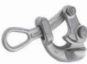
Designed for use when light, compact grip is desired and where conductor damage is not a factor. Gripping pressure of the knurled jaw is applied to 1/4" cable area.
