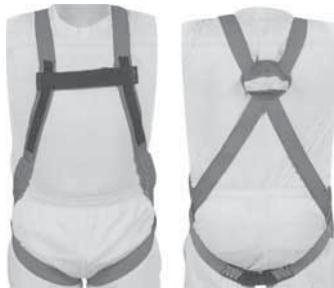
Type 13 nylon webbing construction. Features orange upper and black lower section, reinforced web looper dorsal attachment for half-hitching a shock absorbing lanyard, and step-in leg straps. Meets ANSI requirements.
