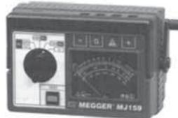
Features (4) different test voltages: 100, 250, 500 and 1000 DCV for spot and step voltage testing. Measures insulation resistance up to 2000 MW, and an ohm range to 5000 W. Guard terminal to eliminate surface leakage current.
