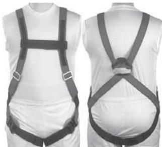
Full body harness features leg straps with Quick Connect Buckles, hook and loop chest strap that meets ANSI requirements, web dorsal loop attachment, and friction buckles mounted on vertical shoulder strap for height adjustment. Designed with minimal amount of metal above the waist.
