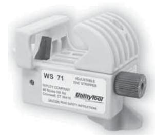
Used for end stripping 600V secondary cable. Can accommodate a cable range of 1/2" to 1.3" OD. Features bright color for easy visibility and quick release adjustment to simplify sizing. Constructed of impact resistant and lightweight polymer material.
