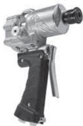
Impact and temperature resistant replaceable polymer grip designed to dissipate heat from the cast handle. Features built-in hydraulic check valve, large lifting eye for easy and secure storage, and longer and wider trigger for improved control with insulated gloves 7/16" hex, 1/2" drive size and 4-12 GPM flow range.
