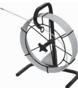
Features sturdy, powder coated, steel tube frame with a 16" diameter storage basket. Up to 400 ft. of rod can be stored in basket. Light adjustable brake prevents the rod from reeling out of the basket under its own tension.
