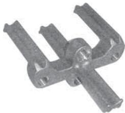
For connecting ground cables together. Aluminum alloy construction. Features (4) terminal positions tapped for use with 5/8"-11 NC threaded grounding ferrules, and stress relief grounding cable pads. Tested for 43KA @ 15 cycles.
