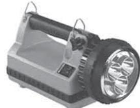
Features high-impact ABS thermoplastic housing, rubberized impact bumper, lens ring, and cushioned-grip handle. Toggle switch for use with gloves. Includes (3) shockproof C4 LEDs with a 50,000 hour lifetime. 615 Lumens. Orange.
