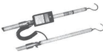
For circuit potential and URD cable testing applications. Attaches to (2) 1-1/4" dia. x 16" L fiberglass sticks. Universal female splines on one end, (2) 2" dia. conductor hooks on other end. Features LCD display in nearest 100V, automatic shutoff, low battery indicator, and coiled, self-retracting cable. Includes 9V battery and plastic case.
