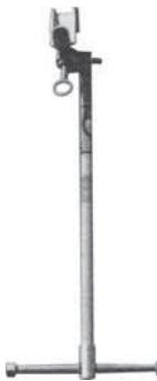
Extends length of existing mechanical jumpers. Supports (2) jumpers while isolating connection from other potentials. Can also be used as parking stand or ground jumper holder. Features non-conductive fiberglass shaft and solid copper contact bar.
