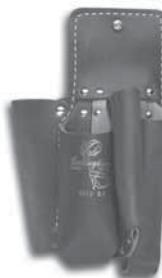
Double back holsters stay rigid after years of use to ensure easy tool removal from pockets. Features pockets that are riveted to a thick layer of leather with another leather layer sewn over the rivet heads, with plastic stiffener sandwiched in between.
