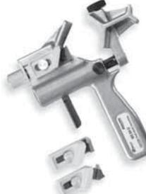
Universal tool for end stripping or mid span stripping of outer jackets or insulating material. The end stripping and mid span stripping are done with different blades and allow for dual position of the jaw for cable sizes 1/2" to 2-1/2"
