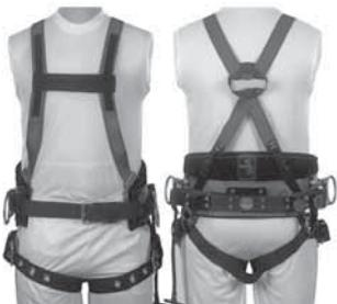
A lightweight full float body belt with an extra wide back support. The back pad is 8" of continuous firm cushion lined with durable brushed leather. The 1-3/4" waist strap is 6-ply neoprene impregnated nylon with 9 adjustment holes.
