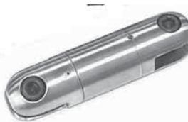
Constructed with a thrust bearing for tensile load and a radial bearing for bending load. High safe working load combined with a compact design. All sizes incorporate an oil seal and are manufactured from high strength stainless steel.
