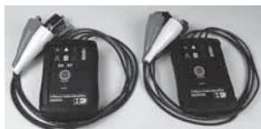
Identifies correct phases on long lengths of de-energized and discharged overhead and underground cables. Includes sender and receiver designed to be hand held with or without gloves.
