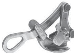
Designed with a round inside-jaw contour for maximum contact to minimize conductor damage. Includes latch to prevent grip from falling in case of jaw disengagement from cable.
