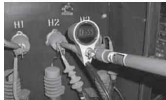
Multi-function design for use on primary or secondary voltages or capacitive test points. Features 3/4" backlit LCD meter, 5-position selector switch, shielded housing and interconnect cable, and impact/wear resistant probes. Accurate to  $\pm 1\%$ .
