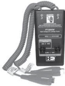
Portable, general purpose dual voltage leakage tester designed to test primary distribution voltage or secondary voltage equipment for faults or high leakage currents. Use only on cable or equipment verified to be both de-energized and discharged. Can be set to either 500VDC or 5000VCD.
