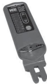
Detects voltages 10" or greater from source and most elbow test points. Features rechargeable battery with quick recharge, (9) standard voltage ranges from 120 VAC up to 500 kVAC, and loud beeper and LED lights to indicate voltage.
