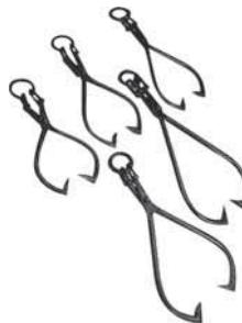
For pulling or skidding material along ground. Constructed of 1" round high-carbon steel stock. Features heavy up-set hammer-forged points with flattened sides at pivot. Includes ring.
