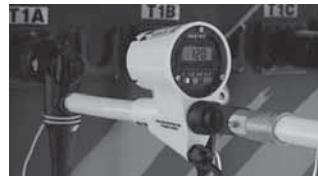
For use with 208V to 69kV distribution systems (direct contact) or 69kV to 800kV transmission systems (non-contact; degree position only). Features reference probe (transmitter) and meter probe (receiver) with color-coded LED indicators and 5-position selector switch. Impact- and wear-resistant. Meter probe features backlit digital display.
