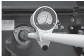
For proximity or direct contact use on overhead or underground systems. Detects 0 to 40kV line to ground; 0 to 69kV phase to phase. Features analog scale, 5-position selector switch, internal overload protection, and backlight for use in low light. Water resistant. Includes carrying case.
