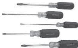
Features precision-machined black phosphated tips, and cushioned grip. Handle marked with size, type and length. Rust resistant chrome plated finish. Includes 3/16" x 6" and 1/4" x 6" cabinet, 1/4" x 4" and 5/16" x 6" keystone, and #2 x 4" Phillips drivers.
