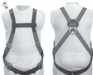
Universal sized full body harness features hook and loop chest strap, shoulder strap adjustment, interlocking leg buckles, and dorsal dee ring.
