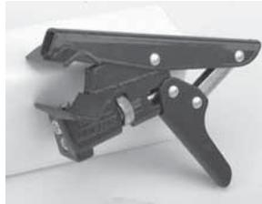
For mid-span and end termination. Strips TW, THW, THWN, THHN and similar single-layer insulation.
