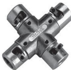
For use with 600-volt secondary cable. Strips 45 mil to 110 mil insulation with choice of square cut or chamfer cut. Guarded blades ensure safe, precise stripping with no conductor damage. Bushings change with hex wrench.
