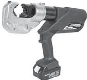
12 ton. Features two speed pump, pressure monitoring system, automatic retraction stop, LED light, and pistol grip. 24,000 lbs. crimping force. Includes (2) 18V lithium ion batteries, battery charger and carry case. Measures 16-1/4" L x 2-7/8" W x 12-1/2" D.
