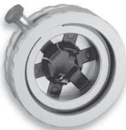
For use on .650 to 1.875 in. cable OD and is able to chamfer 15 to 35 KV cable. Creates a 45° bevel, approximately .125" long. Tool adjusts easily to fit different cable insulations.
