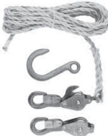
Blocks with standard snap hooks. Includes 25' of 3/8" rope, block with snap hook and a detachable forged anchor hook on one end, and block with eye and rope tie-off on other end. Not occupational protective hooks and not for human support. Maximum safe load 750 Lbs.
