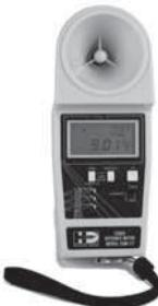
Measures cable sag, cable height distance and overhead clearance of conductors. Utilizes ultrasonic signals to determine the height of over cable up to 75 ft. Features 3-button operation and low battery indicator.
