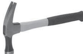
Elongated neck and narrow striking face for use in boxes and other confined spaces. Features long straight claws, fiberglass handle with flared end, and cushioned grip.
