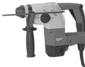
Compact design for use in concrete drilling, overhead work and confined space applications. Features 7 Amp reversible motor, met gear case, anti-vibration system, two-finger trigger, rotating brush plate, 10-ft. cord and soft grip D-handle. Three operating modes: hammer drill; drill and chipping. 1" solid bit capacity; 2-1/2" thin wall core bit capacity. 120V AC.
