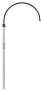
Used to withdraw injured worker from hazardous areas, confined spaces, vaults or near electrical cabinets and switch gear. Features foam filled, fiberglass reinforced handle for electrical insulation. Includes coated heat treated body hook with 18" opening.
