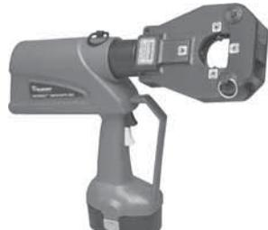
For use on copper, aluminum, compressed, compact, stranded, solid and flex conductors. Features rotating head, locking latch pin, audible pop-off valve, trigger guard and safety lanyard connection. Measures 17.6" L x 3.7" W x 13.9" H. Includes (2) 18V Ni-MH batteries, battery charger, lanyard and carry case.
