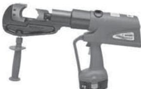
Allows user to interchange different cutting blades customized for the application. Features C-head cutter and 355° swivel. For use on ACSR, guy strand, ground rod, rebar, soft steel bolts, copper and aluminum.
