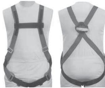
Type 13 nylon webbing construction. Features orange upper and black lower section, Velcro® chest strap, interlocking leg strap buckles with leather chafes, web dorsal loop attachment, and friction buckle for height adjustment. Meets ANSI requirements.
