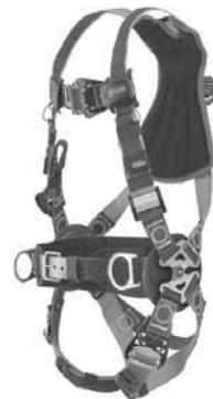
Features Kevlar web loop back pad, 10,000 lb. tensile strength webbing with permanent fire retardant (FR) properties, and leather insulators under all metal hardware. Universal (L/XL). Rated to 400 lbs.
