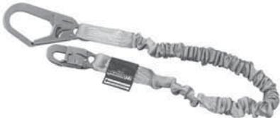
Contracts 6 ft to 4 ft to reduce tripping, snagging or dragging. Specially-woven shock-absorbing inner core smoothly expands to reduce fall arrest forces. Flag released after fall. Features locking snap hook harness and locking rebar hook anchorage connection.
