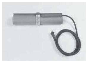
Wrap blanket around PVC, secure with hook and loop strap. Built-in stiffeners keep blanket tight to PVC surface. Heavy-duty cord and thermostat for long life. Over 300° F. 120 VAC.
