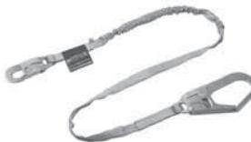
Specially-woven shock-absorbing inner core smoothly expands to reduce fall arrest forces. Warning flag alerts fall. Heavy duty tubular outer jacket serves as back-up lanyard.
