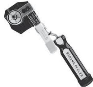
For use in removing semi-con URD cable shield without damaging underlying insulation. Scores circumference and length. Features spring-loaded blade assembly and Teflon coated cable guide.
