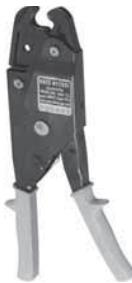
For installation of 5/8" Insulink™ and Linkit™ service entrance connectors with single crimp per end. Features full cycle ratchet and cam mechanism, forged steel jaws, stainless steel indentor, and spring loaded comfort grip handles. 50-lbs. hand force develops 6000-lbs. crimp force.
