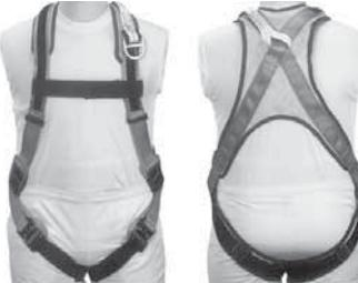
Full body harness with Kevlar® mesh shell that is designed to breathe. Features foam padded shoulder and leg pads, hook and loop chest strap that meets ANSI requirements, Quick Connect buckles, and 18" dorsal pigtail with small dee ring to attach a 4-1/2' shock absorbing lanyard.
