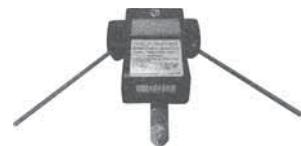
For use in verifying neutral position on regulators. Measures 0 to 2000 Volts in 1V increments. Features LCD display, lighted meter switch, low battery indicator, female universal spline for use with hot sticks, and removable knurled contact electrodes to aid conductor contact. Includes 9V battery, carry case and instructions.
