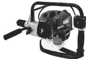
Features 25.4cc engine, electronic ignition, throttle lockout, spark-arresting muffler, ergonomic front handle, and 1/2" keyless chuck. Reversible. 17:1 to 1 gear reduction ratio. 10.7 lbs.
