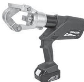
For use on copper and aluminum lugs and splice through 1000 kcmil. Indent style dieless design. Features pressure monitoring system, automatic retraction stop, LED light, and pistol grip. 24,000 lbs. crimping force. Includes (2) 18V lithium ion batteries, 120V battery charger and carry case.
