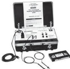
For checking resistance in electric utility applications. Applies direct current across test specimen. Features ball-stud terminals, (2) troubleshooting probes, and self-test cable. Includes videotape demonstration, instruction manual and self-contained carry case.
