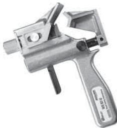
For mid-span stripping of high density outer jackets or insulating material on cables from 1/2" to 1-1/2" OD. Features spring-loaded jaw, micro-adjustable blade, and self feeding design.
