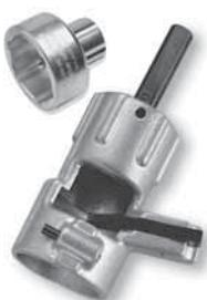
Used for 15 to 46 KV cables with .900 to 2.030 in. cable OD. Strips XLPE, polyethylene and EPR insulation and provides precision stripping with no conductor damage. Features guarded cutting blade and rotating stop bar. Includes adapter for use of the SW2 ratchet wrench.
