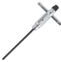
For use with 200A bushing inserts with internal hexagon socket drive. Features adjustable T-handle, 1" square socket drive, 7/8" hexagon for wrench, and Penta head.
