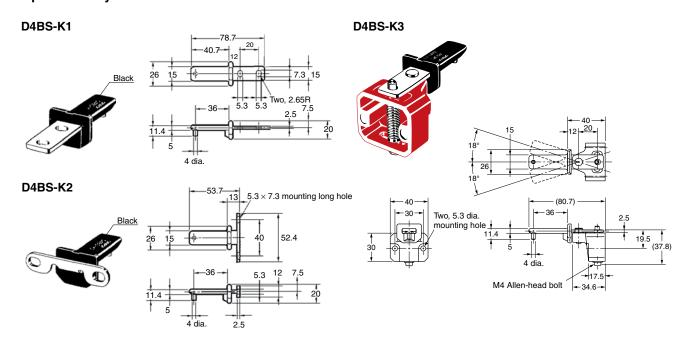
Note: Unless otherwise specified, a tolerance of ±0.4 mm applies to all dimensions.
