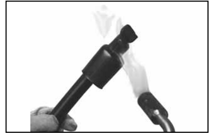
2. Beginning at closed end apply heat, blue thermochromatic lines will begin to disappear at 150° C. Gradually, move heat source to open end and around cap. Once lines are no longer visible and adhesive flows out of open end, discontinue heating.
