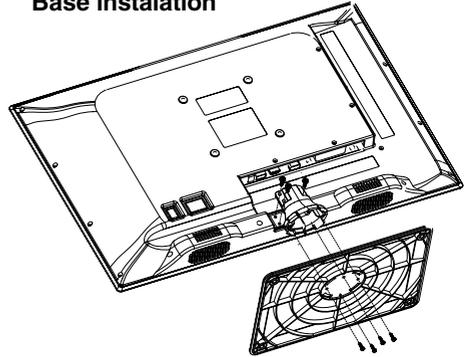
Cover a flat stable surface with a soft cloth. Place the TV unit facedown on the cloth. First align the base with the holes on the back of the unit and fix it with 4 PB4\*14mm screws. Then match the holes in the stand with the fixing pins in the bottom of the base. Fasten with 3 BB3\*8mm screws.
