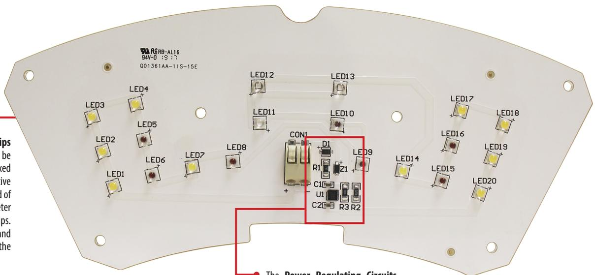
The Power Regulating Circuits ensure all the chips and boards are receiving the same voltage to produce a consistent intensity and maintain the spectral quality.
