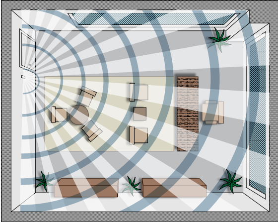
PIR and Ultrasonic coverage patterns shown above.
