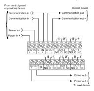
The Remote Relay Module (FSRRM24) is one component of the system that sets E-FSC apart from other panels in its class. This module has five Form
