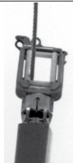
Center wireholder, used alone, permits single-phase lifts.
