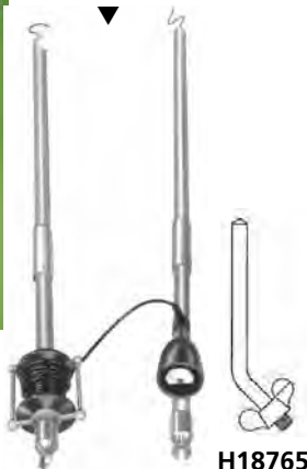
Extension Resistors, as installed
