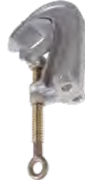
C6000375 Aluminum body, Serrated jaws, Bronze eyescrew with Acme threads, Dual drilled for 3/8"-11 UNC threaded ferrule
