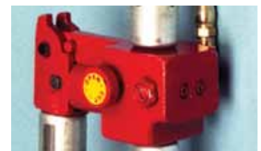
Single control knob selects direction. Notice: When storing tool, be sure to relieve hydraulic pressure by turning knob to the Open position.
