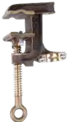
C6002232 Bronze body, Serrated jaws, Bronze eyescrew with Acme threads, Drilled for 5/8-11 UNC threaded ferrule or T6003196, Tapped for 5/8-11 UNC threaded ferrule
