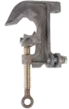
T6000658 Aluminum body, Smooth jaws, Bronze eyescrew with Acme threads, Drilled for 5/8-11 UNC threaded ferrule
