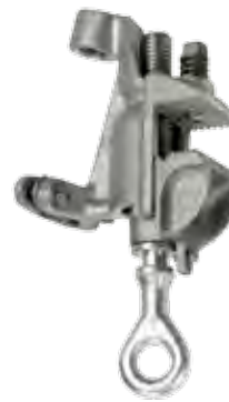
C6001735 Aluminum body, Serrated jaws, Bronze eyescrew with fine threads, Tapped for 5/8-11 UNC threaded ferrule
