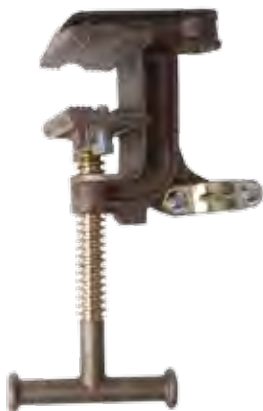
C6002231 Bronze body, Serrated jaws, Bronze T-handle with Acme threads, Drilled for 5/8-11 UNC threaded ferrule or T6003195, Tapped for 5/8-11 UNC threaded ferrule
