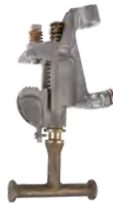
T6001798 Aluminum body, Serrated jaws, Bronze T-handle with Acme threads, Tapped for 5/8-11 UNC threaded ferrule
