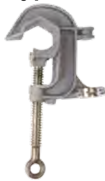
C6002255 Aluminum body, Smooth jaws, Bronze eyescrew with Acme threads, Tapped for 5/8-11 UNC threaded ferrule
