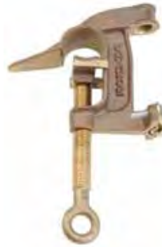
C6002271 Bronze body, Smooth jaws, Bronze eyescrew with fine threads, Tapped for 5/8-11 UNC threaded ferrule
