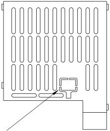
BC215 Finger-Safe Cover Cut Out Tab (3 Places) to Access Field Terminals. (For Shunt Wound Motors Only.)
