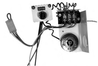
CP-PE-HOA-3POS HOA switch – for field installation
