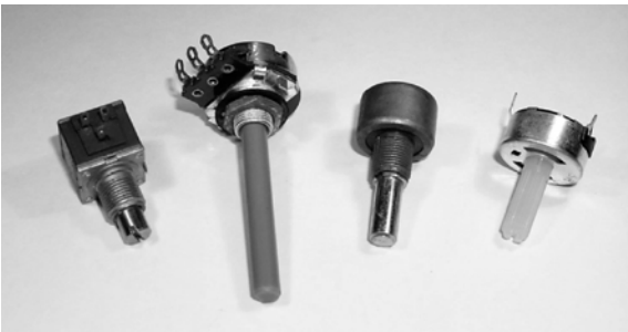
Figure 2.20 A selection of common types of carbon and wirewound variable resistors/potentiometers
