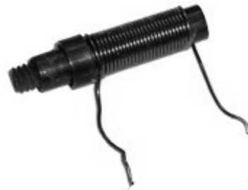
Figure 2.43 An adjustable ferrite cored inductor
