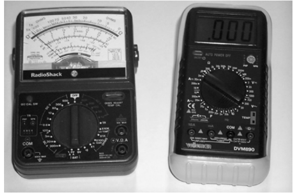
Figure 14.6 Typical analogue (left) and digital (right) multimeters
