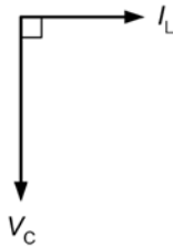
Figure 4.7 Phasor diagram for a pure capacitor
