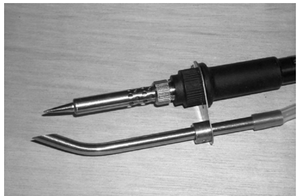
Figure 19.17 Fume extraction facility which can be added to a temperature controlled iron when necessary
