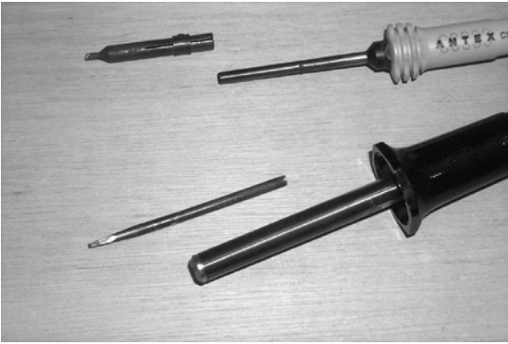
Figure 19.18 Two different types of bit fitted to small soldering irons
