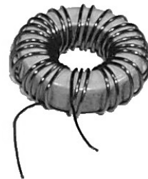
Figure 2.35 A practical coil contains inductance and resistance
