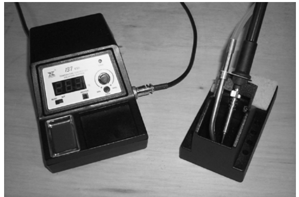
Figure 19.16 A modern temperature-controlled soldering station with ESD and fume extraction facilities
