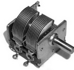
Figure 2.34 An air-spaced variable capacitor. This component (used for tuning an AM radio) has two separate variable capacitors (each of 500 pF maximum) operated from a common control shaft.
