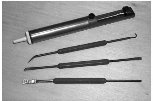
Figure 19.27 A variety of desoldering tools (including desoldering pump and wire brush)
