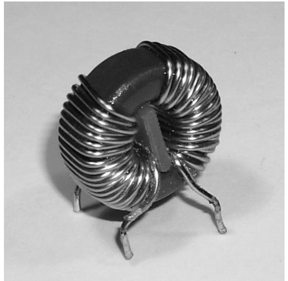
Figure 4.23 This small 1:1 ratio toroidal transformer forms part of a noise filter connected in the input circuit of a switched mode power supply. The transformer is wound on a ferrite core and acts as a choke, reducing the high-frequency noise that would otherwise be radiated from the mains supply wiring
