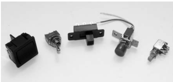
Figure 1.19 Various types of switch. From left to right: a mains rocker switch, an SPDT miniature toggle (changeover) switch, a DPDT slide switch, an SPDT push-button (wired for use as an SPST push-button), a miniature PCB mounting DPDT push-button (with a latching action).
