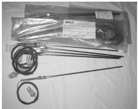
Figure 16.2 A selection of thermocouple probes
