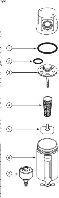
**Model 5200 Internal Float Drain Available (Item #7)** To be used for pressures from 30 psi to 175 psi and from 40°F to 120°F. To order filter with float drain assembled, add suffix "F" to filter model number.
