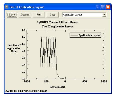
Figure 83. Application layout, combining the spray block deposition (Figure 84) to 630 ft upwind of the edge of the application area (at 0 ft) and the downwind deposition to 1000 ft.
