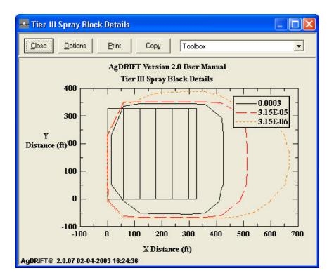
Figure 95. Spray Block Details contour results for ASAE S-572 Fine to Medium drop size distribution with zero swath displacement. Deposition is in ozf/ft<sup>2</sup>.
