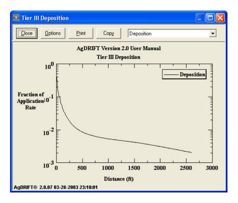
Figure 63. ASAE S-572 Medium to Coarse drop size distribution deposition curve.
