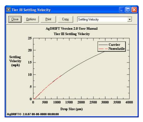
Figure 82. Settling velocity as a function of drop size, for the carrier and nonvolatile fraction assumed. The two curves will be different only if specific gravity is different.
