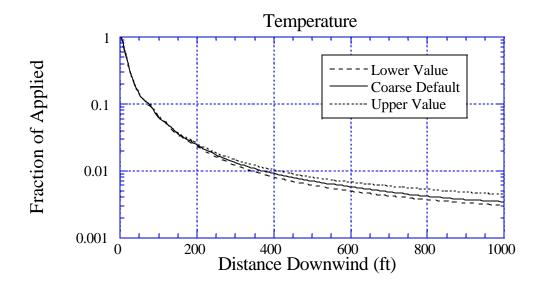
Figure 73c. Sensitivity of deposition to a 10% variation in Temperature: the solid curve is for the default value of 86.0°F; the long-dashed curve is for a lower value of 77.4°F; and the dotted curve is for an upper value of 94.6°F. BCPC Medium to Coarse drop size distribution.
