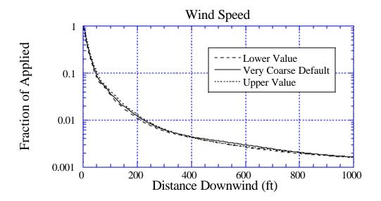
Figure 75d. Sensitivity of deposition to a 10% variation in Wind Speed: the solid curve is for the default value of 10 mph; the long-dashed curve is for a lower value of 9 mph; and the dotted curve is for an upper value of 11 mph. BCPC Coarse to Very Coarse drop size distribution.
