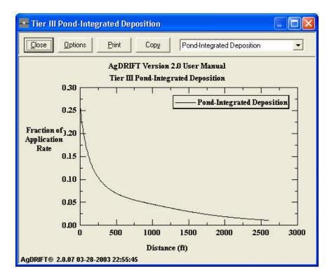
Figure 61. Plot of the pond-integrated deposition for the ASAE S-572 Very Fine to Fine drop size distribution aerial application.
