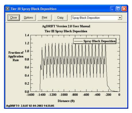
Figure 84. Spray block deposition pattern, measured from the edge of the application area (at 0 ft) upwind into the spray block (20 flight lines assumed in this example).
