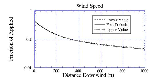
Figure 75a. Sensitivity of deposition to a 10% variation in Wind Speed: the solid curve is for the default value of 10 mph; the long-dashed curve is for a lower value of 9 mph; and the dotted curve is for an upper value of 11 mph. BCPC Very Fine to Fine drop size distribution.
