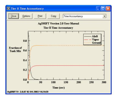
Figure 88. Total accountancy of the released tank mix material, for the most downwind flight line, as a cumulative function of distance.
