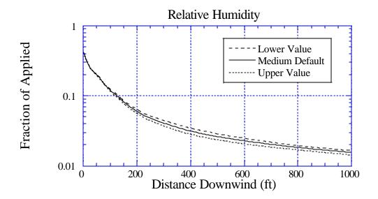
Figure 71b. Sensitivity of deposition to a 10% variation in Relative Humidity: the solid curve is for the default value of 50%; the long-dashed curve is for a lower value of 45%; and the dotted curve is for an upper value of 55%. BCPC Fine to Medium drop size distribution.
