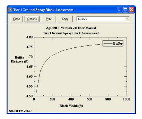
Figure 18. Spray Block Assessment for the Low Boom ASAE S-572 Very Fine to Fine drop size distribution. The 0 ft location (on the vertical axis) locates the edge of the application area.
