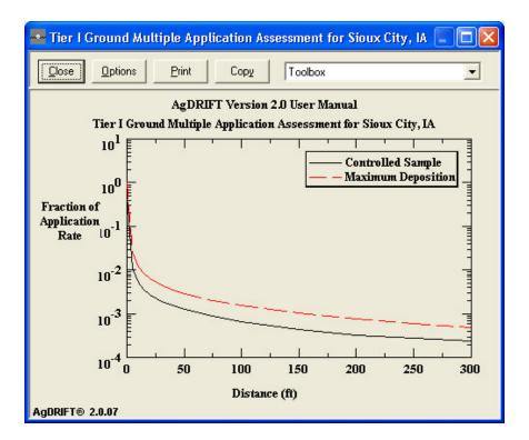
Figure 24. Multiple Application Assessment for the Low Boom ASAE S-572 Very Fine to Fine drop size distribution in Tier I for Sioux City, IA. The curves are the average multiple application deposition pattern (including zero deposition effects when the wind is blowing upwind of the spray block) and the maximum deposition pattern recovered across the selected wind speed range. Ten events per year assumed.
