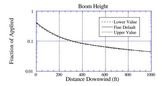
Figure 68a. Sensitivity of deposition to a 10% variation in Boom Height: the solid curve is for the default value of 10 ft; the long-dashed curve is for a lower value of 9 ft; and the dotted curve is for an upper value of 11 ft. BCPC Very Fine to Fine drop size distribution.
