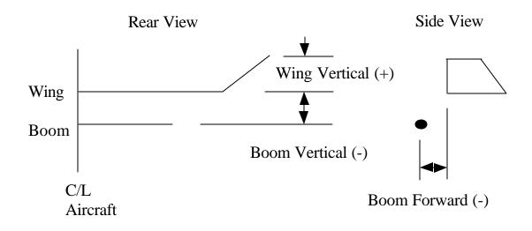
Figure 30. Schematic of aircraft wing and boom details.
