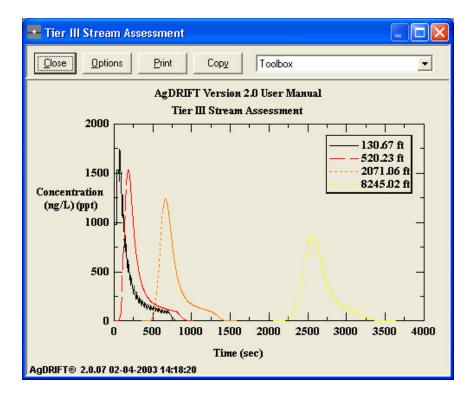
Figure 66. Time profiles of active spray material deposited to a stream at four distances identified on the plot.
