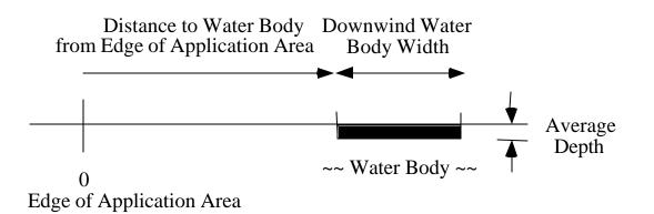
Figure 13. Cross section of the water body size and downwind location relative to the edge of the application area.
