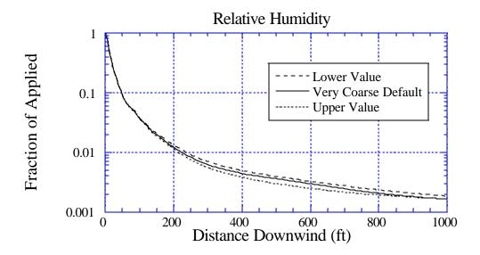
Figure 71d. Sensitivity of deposition to a 10% variation in Relative Humidity: the solid curve is for the default value of 50%; the long-dashed curve is for a lower value of 45%; and the dotted curve is for an upper value of 55%. BCPC Coarse to Very Coarse drop size distribution.
