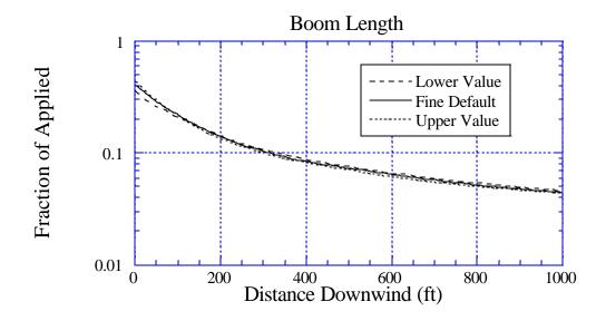
Figure 69a. Sensitivity of deposition to a 10% variation in Boom Length: the solid curve is for the default value of 76.3%; the long-dashed curve is for a lower value of 68.7%; and the dotted curve is for an upper value of 83.9%. BCPC Very Fine to Fine drop size distribution.
