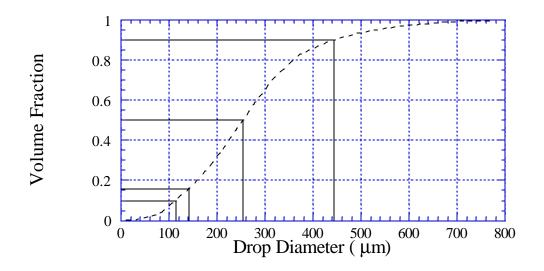
Figure 62. Cumulative spray volume for the ASAE S-572 Fine to Medium drop size distribution, plotted as a function of the average drop diameter in each size class, and the locations for  $D_{v0.1}$ ,  $D_{v0.5}$ ,  $D_{v0.9}$ , and 141  $\mu$ m.
