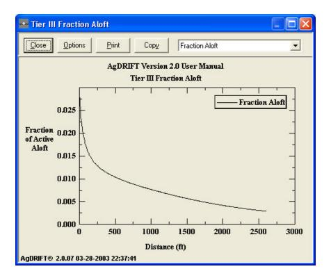
Figure 51. Fraction Aloft for the ASAE S-572 Medium to Coarse drop size distribution and all model defaults.
