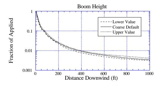
Figure 68c. Sensitivity of deposition to a 10% variation in Boom Height: the solid curve is for the default value of 10 ft; the long-dashed curve is for a lower value of 9 ft; and the dotted curve is for an upper value of 11 ft. BCPC Medium to Coarse drop size distribution.
