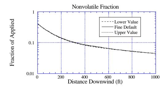
Figure 70a. Sensitivity of deposition to a 10% variation in Nonvolatile Fraction: the solid curve is for the default value of 0.03; the long-dashed curve is for a lower value of 0.027; and the dotted curve is for an upper value of 0.033. BCPC Very Fine to Fine drop size distribution.
