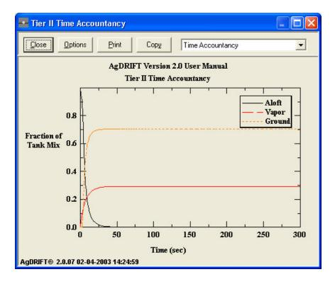
Figure 87. Total accountancy of the released tank mix material, as a cumulative function of time after release.
