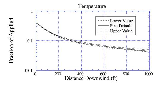
Figure 73a. Sensitivity of deposition to a 10% variation in Temperature: the solid curve is for the default value of 86.0°F; the long-dashed curve is for a lower value of 77.4°F; and the dotted curve is for an upper value of 94.6°F. BCPC Very Fine to Fine drop size distribution.
