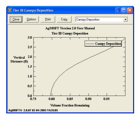
Figure 86. Canopy deposition profile, for an Optical Aspen canopy with a height of 3 ft and a LAI of 0.1. Aircraft boom height is 10 ft.
