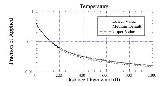
Figure 73b. Sensitivity of deposition to a 10% variation in Temperature: the solid curve is for the default value of 86.0°F; the long-dashed curve is for a lower value of 77.4°F; and the dotted curve is for an upper value of 94.6°F. BCPC Fine to Medium drop size distribution.
