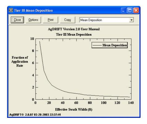
Figure 50. Mean Deposition within the spray block as a function of Swath Width.
