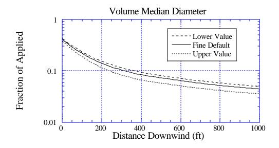
Figure 74a. Sensitivity of deposition to a 10% variation in Volume Median Diameter D<sub>r0.5</sub>: the solid curve is for the default value of 119.23 μm; the long-dashed curve is for a lower value of 107.31 μm; and the dotted curve is for an upper value of 131.15 μm. BCPC Very Fine to Fine drop size distribution.
