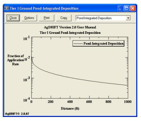
Figure 9. A plot of the Tier I pond-integrated deposition for the Low Boom ASAE S-572 Very Fine to Fine drop size distribution.
