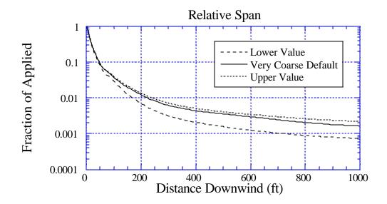
Figure 72d. Sensitivity of deposition to a 10% variation in Relative Span: the solid curve is for the default value of 1.211; the long-dashed curve is for a lower value of 1.090; and the dotted curve is for an upper value of 1.332. BCPC Coarse to Very Coarse drop size distribution.
