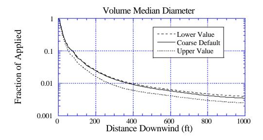
Figure 74c. Sensitivity of deposition to a 10% variation in Volume Median Diameter  $D_{0.5}$ : the solid curve is for the default value of 352.98  $\mu$ m; the long-dashed curve is for a lower value of 317.68  $\mu$ m; and the dotted curve is for an upper value of 388.28  $\mu$ m. BCPC Medium to Coarse drop size distribution.
