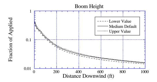
Figure 68b. Sensitivity of deposition to a 10% variation in Boom Height: the solid curve is for the default value of 10 ft; the long-dashed curve is for a lower value of 9 ft; and the dotted curve is for an upper value of 11 ft. BCPC Fine to Medium drop size distribution.
