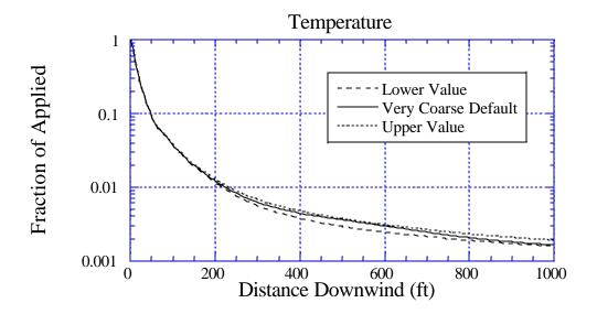
Figure 73d. Sensitivity of deposition to a 10% variation in Temperature: the solid curve is for the default value of 86.0°F; the long-dashed curve is for a lower value of 77.4°F; and the dotted curve is for an upper value of 94.6°F. BCPC Coarse to Very Coarse drop size distribution.
