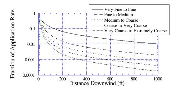
Figure 2. Deposition as a function of distance for the five ASAE S-572 threshold categories. These curves represent the upper range of deposition as a fraction of the nominal application rate for the Very Fine, Fine, Medium, Coarse, and Very Coarse atomization regimes. Simulation results assume a 20-swath field application
