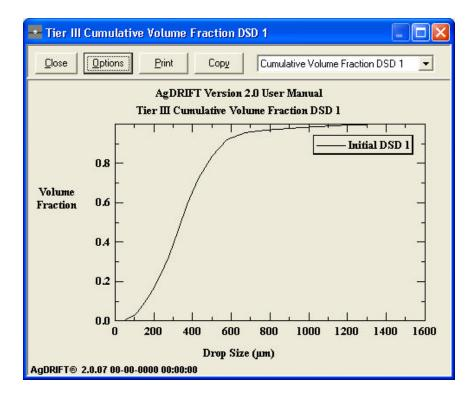
Figure 46. A cumulative plot of the ASAE S-572 Medium to Coarse drop size distribution.
