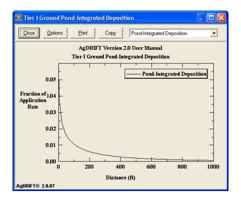
Figure 59. Plot of the pond-integrated deposition for the High Boom (ULV) ground sprayer application.
