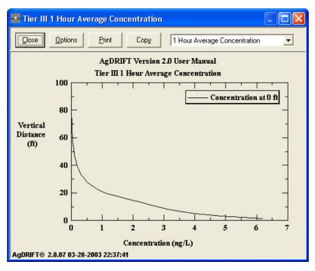
Figure 48. One hour average concentration through a flux plane positioned at the edge of the application area for the same conditions as Figure 47.
