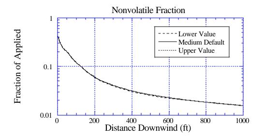
Figure 70b. Sensitivity of deposition to a 10% variation in Nonvolatile Fraction: the solid curve is for the default value of 0.03; the long-dashed curve is for a lower value of 0.027; and the dotted curve is for an upper value of 0.033. BCPC Fine to Medium drop size distribution.
