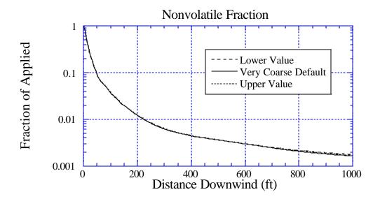
Figure 70d. Sensitivity of deposition to a 10% variation in Nonvolatile Fraction: the solid curve is for the default value of 0.03; the long-dashed curve is for a lower value of 0.027; and the dotted curve is for an upper value of 0.033. BCPC Coarse to Very Coarse drop size distribution.
