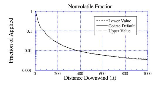
Figure 70c. Sensitivity of deposition to a 10% variation in Nonvolatile Fraction: the solid curve is for the default value of 0.03; the long-dashed curve is for a lower value of 0.027; and the dotted curve is for an upper value of 0.033. BCPC Medium to Coarse drop size distribution.
