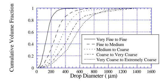
Figure 1. Drop categories used in the definition of the aerial assessment curves. The six drop categories (Very Fine, Fine, Medium, Coarse, Very Coarse, and Extremely Coarse) are based on the nozzle categorization scheme developed in ASAE S-572. The five curves shown here define the upper diameter boundaries of Very Fine, Fine, Medium, Coarse, and Very Coarse atomization regimes.
