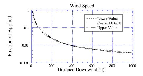
Figure 75c. Sensitivity of deposition to a 10% variation in Wind Speed: the solid curve is for the default value of 10 mph; the long-dashed curve is for a lower value of 9 mph; and the dotted curve is for an upper value of 11 mph. BCPC Medium to Coarse drop size distribution.
