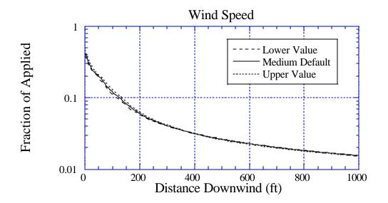
Figure 75b. Sensitivity of deposition to a 10% variation in Wind Speed: the solid curve is for the default value of 10 mph; the long-dashed curve is for a lower value of 9 mph; and the dotted curve is for an upper value of 11 mph. BCPC Fine to Medium drop size distribution.
