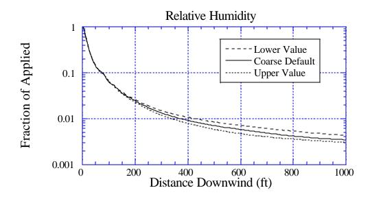
Figure 71c. Sensitivity of deposition to a 10% variation in Relative Humidity: the solid curve is for the default value of 50%; the long-dashed curve is for a lower value of 45%; and the dotted curve is for an upper value of 55%. BCPC Medium to Coarse drop size distribution.
