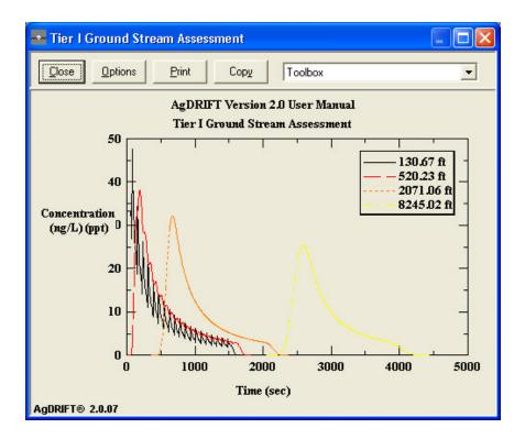
Figure 20. Stream Assessment for the Low Boom ASAE S-572 Very Fine to Fine drop size distribution, with a Turn-Around Time of 30 sec. The 0 ft location locates the center of the spray block in the direction of the sprayer paths.
