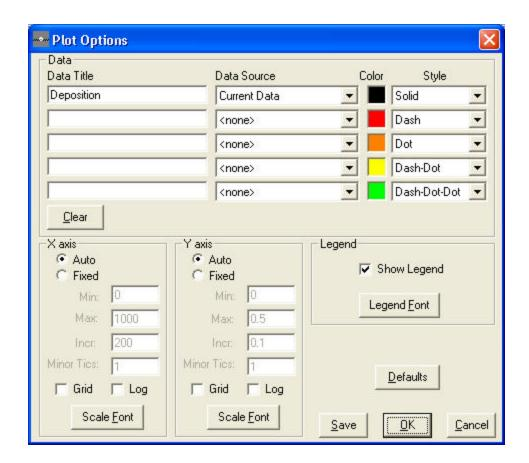
Figure 10. The Plot Options screen reached from the plot screen. Plot Options include additional Data, Color and Style changes, Legend, and manipulation of the X axis (horizontal on the screen) or Y axis (vertical on the screen) with manually selecting the plot size, adding grid or logarithmic appearance, and changing character font.
