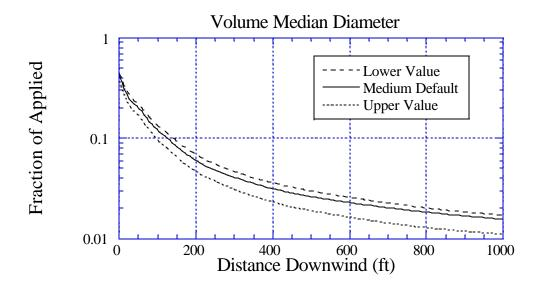
Figure 74b. Sensitivity of deposition to a 10% variation in Volume Median Diameter  $D_{0.5}$ : the solid curve is for the default value of 216.45  $\mu$ m; the long-dashed curve is for a lower value of 194.81  $\mu$ m; and the dotted curve is for an upper value of 238.10  $\mu$ m. BCPC Fine to Medium drop size distribution.
