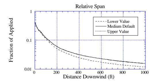
Figure 72b. Sensitivity of deposition to a 10% variation in Relative Span: the solid curve is for the default value of 1.374; the long-dashed curve is for a lower value of 1.236; and the dotted curve is for an upper value of 1.511. BCPC Fine to Medium drop size distribution.
