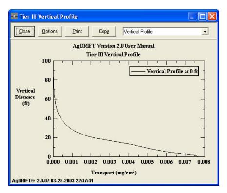
Figure 47. Vertical transport through a flux plane positioned at the edge of the application area for the ASAE S-572 Medium to Coarse drop size distribution and all model defaults.
