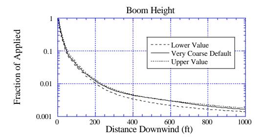
Figure 68d. Sensitivity of deposition to a 10% variation in Boom Height: the solid curve is for the default value of 10 ft; the long-dashed curve is for a lower value of 9 ft; and the dotted curve is for an upper value of 11 ft. BCPC Coarse to Very Coarse drop size distribution.
