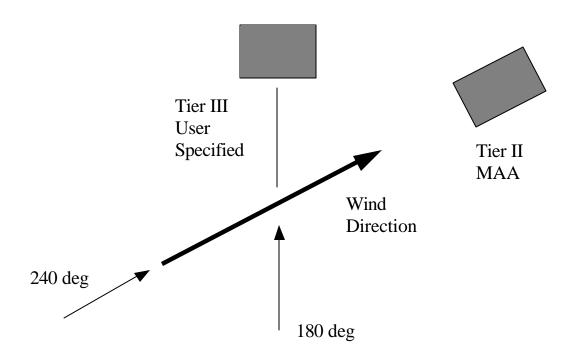
Figure 57. Layout for Multiple Application Assessment in Tier III, where the dominant wind direction blows from 240° (in this example) but the sensitive area (dark square at top) is located 180° to the spray block.
