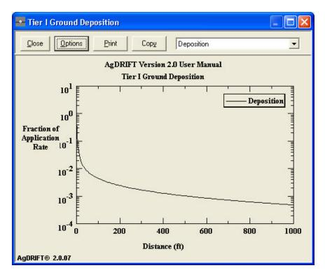
Figure 8. A plot of the Tier I ground deposition for the Low Boom ASAE S-572 Very Fine to Fine drop size distribution. The 0 ft location locates the edge of the application area.
