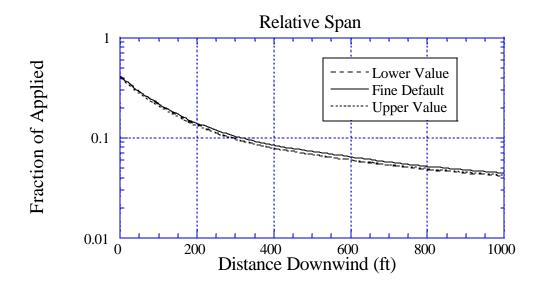
Figure 72a. Sensitivity of deposition to a 10% variation in Relative Span: the solid curve is for the default value of 1.250; the long-dashed curve is for a lower value of 1.125; and the dotted curve is for an upper value of 1.375. BCPC Very Fine to Fine drop size distribution.
