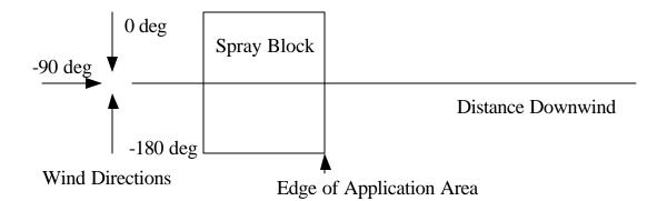
Figure 27. Wind directions (as viewed from above) relative to the spray block and distance downwind.
