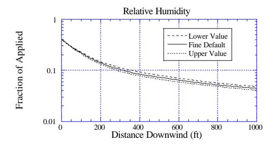
Figure 71a. Sensitivity of deposition to a 10% variation in Relative Humidity: the solid curve is for the default value of 50%; the long-dashed curve is for a lower value of 45%; and the dotted curve is for an upper value of 55%. BCPC Very Fine to Fine drop size distribution.
