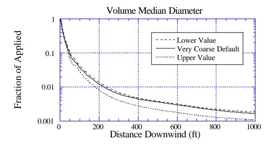
Figure 74d. Sensitivity of deposition to a 10% variation in Volume Median Diameter  $D_{0.5}$ : the solid curve is for the default value of 463.50  $\mu$ m; the long-dashed curve is for a lower value of 417.15  $\mu$ m; and the dotted curve is for an upper value of 509.85  $\mu$ m. BCPC Coarse to Very Coarse drop size distribution.
