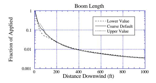
Figure 69c. Sensitivity of deposition to a 10% variation in Boom Length: the solid curve is for the default value of 76.3%; the long-dashed curve is for a lower value of 68.7%; and the dotted curve is for an upper value of 83.9%. BCPC Medium to Coarse drop size distribution.
