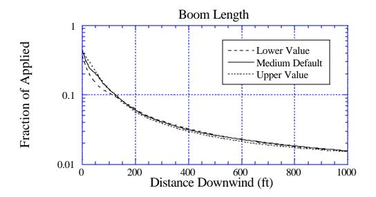
Figure 69b. Sensitivity of deposition to a 10% variation in Boom Length: the solid curve is for the default value of 76.3%; the long-dashed curve is for a lower value of 68.7% and the dotted curve is for an upper value of 83.9%. BCPC Fine to Medium drop size distribution.
