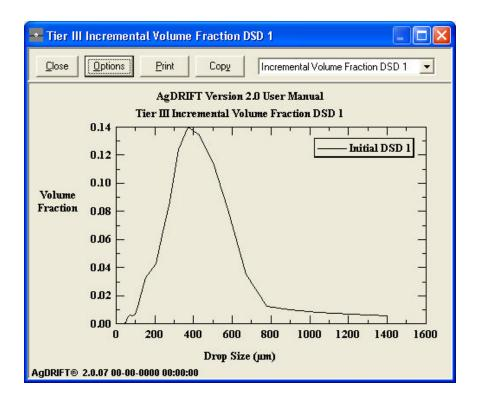
Figure 45. An incremental plot of the ASAE S-572 Medium to Coarse drop size distribution.
