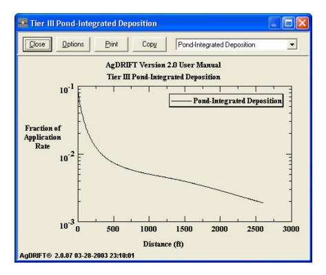
Figure 64. ASAE S-572 Medium to Coarse drop size distribution pond-integrated deposition curve.
