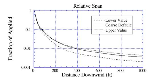
Figure 72c. Sensitivity of deposition to a 10% variation in Relative Span: the solid curve is for the default value of 1.359; the long-dashed curve is for a lower value of 1.223; and the dotted curve is for an upper value of 1.494. BCPC Medium to Coarse drop size distribution.
