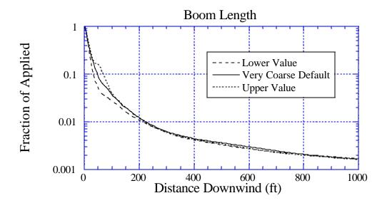
Figure 69d. Sensitivity of deposition to a 10% variation in Boom Length: the solid curve is for the default value of 76.3%; the long-dashed curve is for a lower value of 68.7%; and the dotted curve is for an upper value of 83.9%. BCPC Coarse to Very Coarse drop size distribution.
