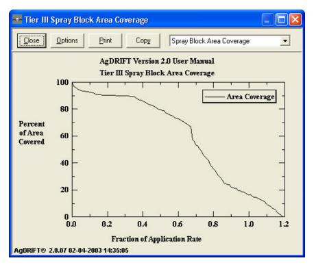
Figure 85. Spray block area coverage, indicating how much area is covered by specified levels of application rate.
