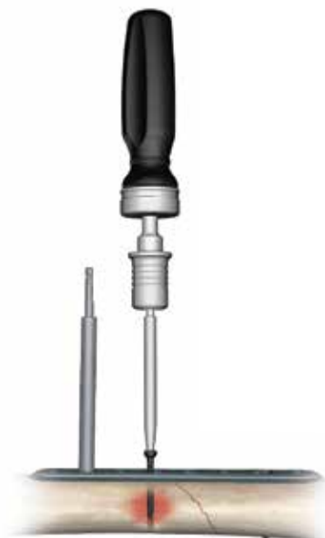
Figure 20 Insert the 4.5 mm non-locking cortical screw using the 3.5 mm hex driver
