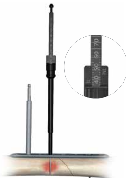
Figure 19 Take the depth reading from the NL line
