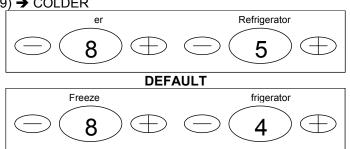
The last FZ Performance Offset value displayed before leaving test 8 will be saved when the refrigerator door(s) is closed.
