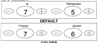
The last FF Performance Offset value displayed before leaving test 7 will be saved when the refrigerator door(s) is closed.
