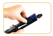
Insert RDO sensor in instrument sensor port.
