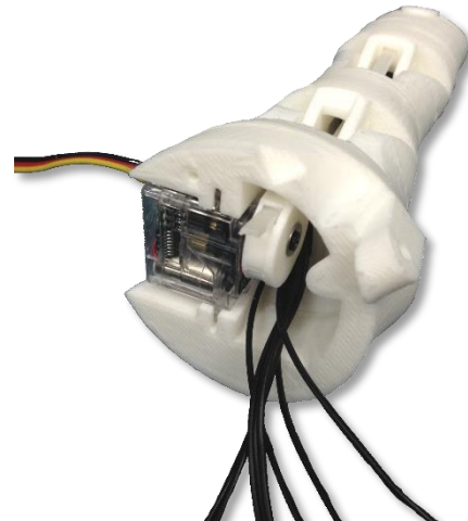
Figure 12: Assembled thumb prior to MC - P Geared Rotator installation, showing servo position
