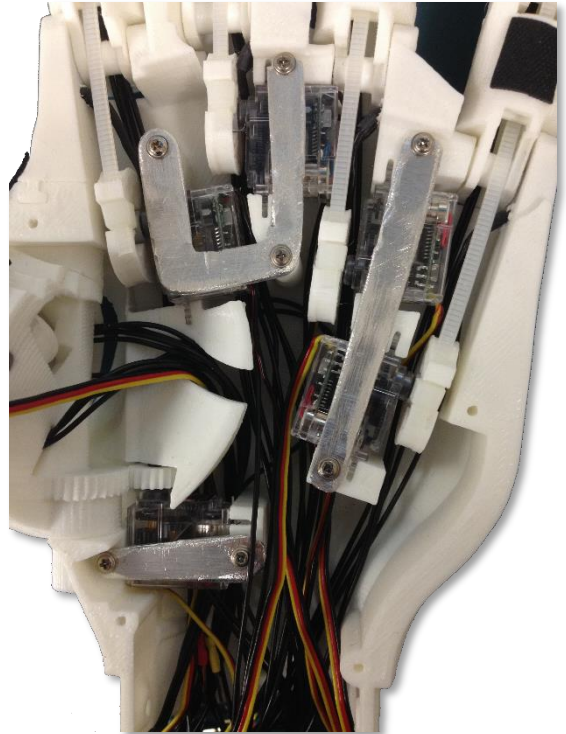
Figure 29: Installation of aluminum servo covers (left hand)
