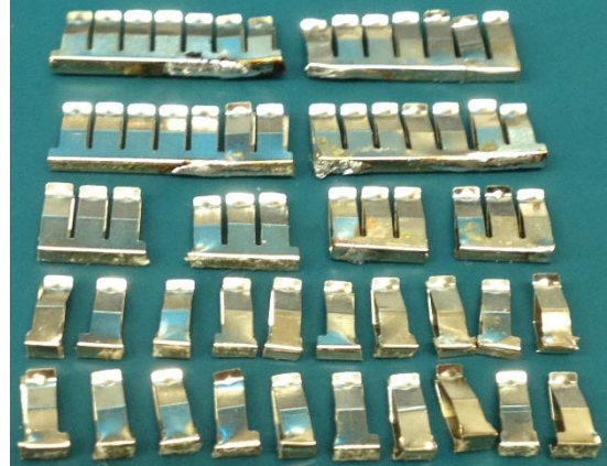
Figure 21: Breadboard clips salvaged from mini breadboard, cut and soldered as necessary
